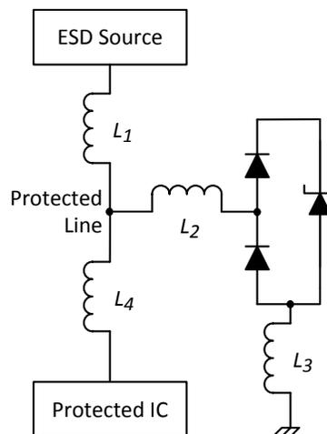
Figure 2-7. PCB Inductance around a Single-channel TVS
