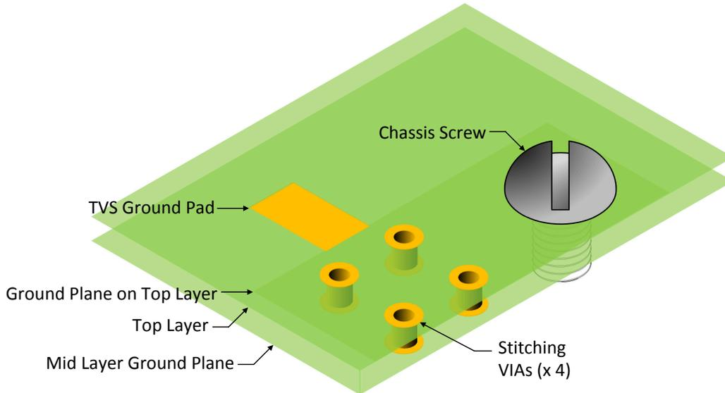
**Figure 2-8. Two Layer PCB - Top Ground Plane Stitched to a Mid-Layer Ground Plane**
