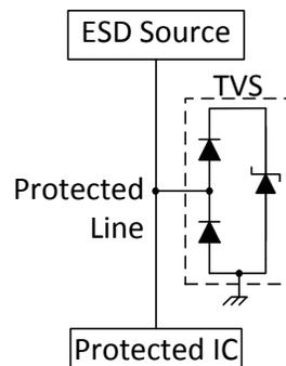
**Figure 1-2. A Typical ESD Protection Scheme**
