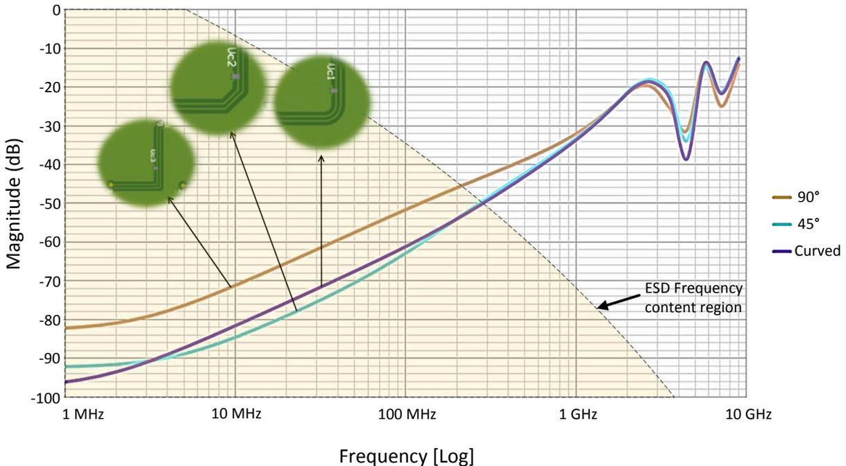
Figure 2-4. Inter-trace Crosstalk with 45°, 90°, and Curved Corners
