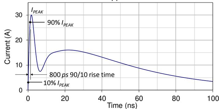
**Figure 1-1. IEC 61000-4-2 Compliant Level 4 (8 kV ESD) Waveform**
