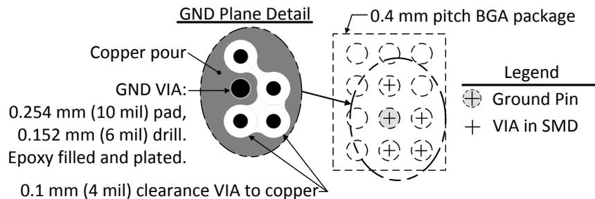
**Figure 2-9. Grounding an Isolated Ground Pin in a BGA Package**
