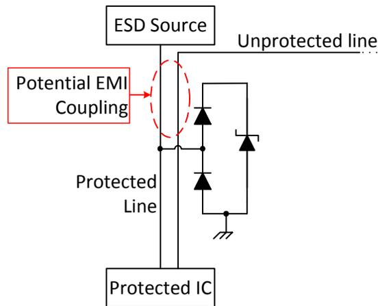
Figure 2-2. EMI Coupling onto an Adjacent Unprotected Trace
