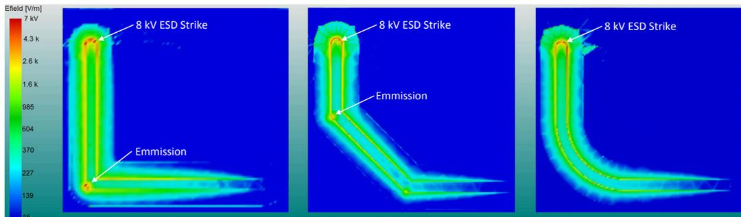
Figure 2-3. Electric Field During an 8 kV ESD Event for Three Different Corner Types
