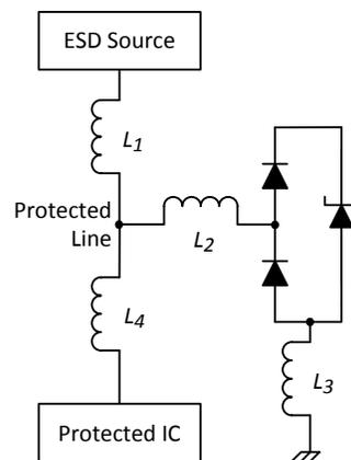
**Figure 2-1. PCB Inductance around a Single-channel TVS**
