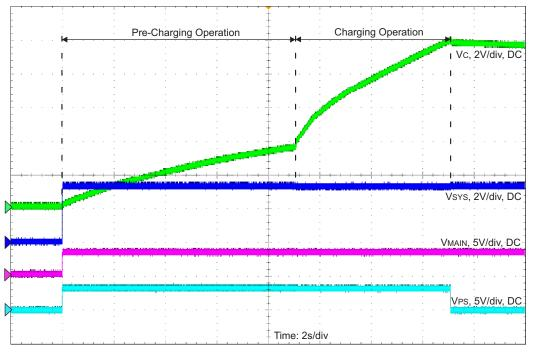
Figure 5. Pre-Charging and Charging of the Backup Capacitor
