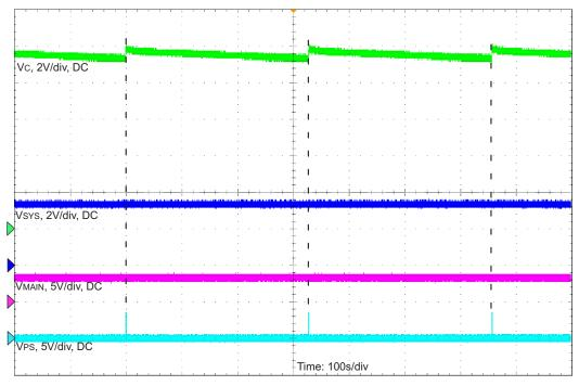
Figure 7. Normal Steady-State Operation
