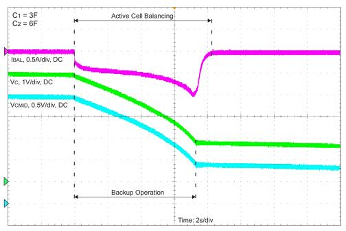
Figure 9. Backup Operation With Enabled Cell Balancing
