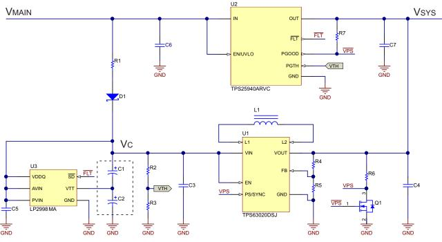
Figure 2. Supercapacitor Backup Power Application Schematic
