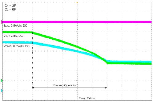
Figure 10. Backup Operation With Disabled Cell Balancing
