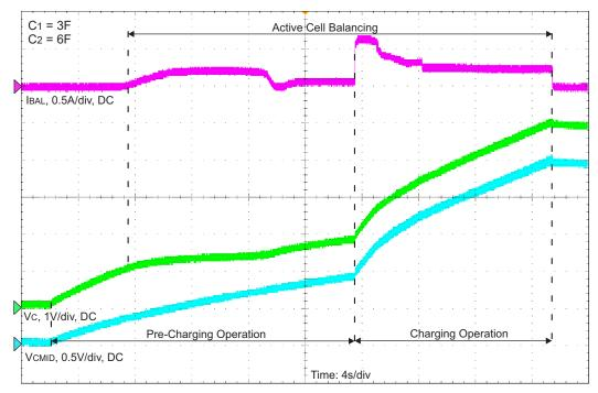
Figure 8. Cell Balancing Operation During Charge Operation
