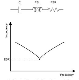
Figure 1. Equivalent Model of Actual Capacitor
