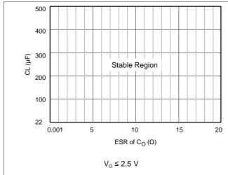
Figure 3. TPS7B67xx-Q1 Stable Region of Output Capacitor
