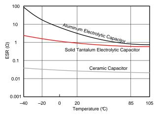
Figure 2. ESR Temperature Characteristics of Different Type Capacitors
