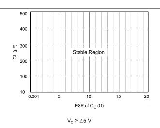
Figure 4. TPS7B67xx-Q1 Stable Region of Output Capacitor
