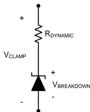
Surge current is generated by the combinational waveform generator outlined in [IEC61000-4-X](#). This current has to be dissipated by the system and more specifically the TVS diode. Since the Flat-Clamp devices have a much lower dynamic resistance the current will be conducted through the device easily while not causing a large clamping voltage for the rest of the system.
