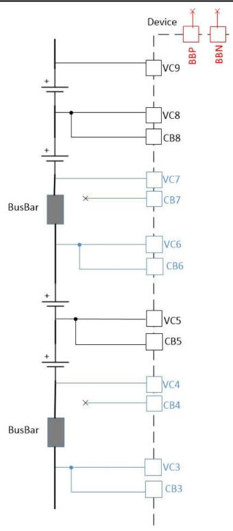
Figure 5-7. Two Bus Bars Connections Using Two Different VC Channel
