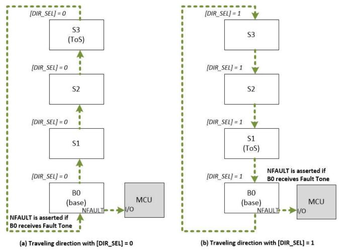
Figure 9-8. Heartbeat or Fault Tone Traveling Direction
