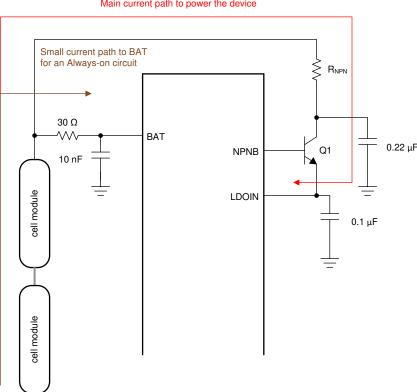
Main current path to power the device
