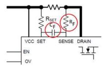
Figure 3. Low-Pass Filter in Current Sense Circuit
