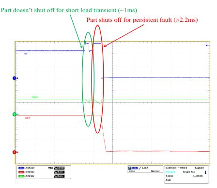
Figure 6. Overcurrent Response (Circuit Breaker) After User-defined Blanking Interval
