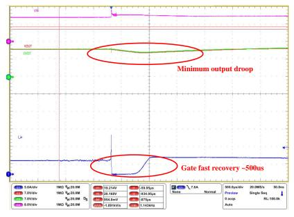
Figure 10. Fast Recovery After Fast-trip
