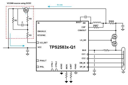
Figure 3. VCONN Sourcing Using the TPS2583x-Q1 DC/DC
