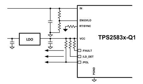
Figure 2. VCONN Source Using an External LDO
