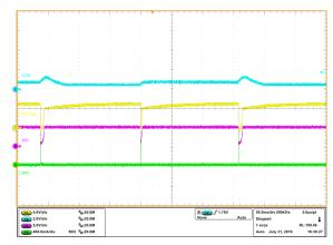
Figure 4. VCC Hiccup, CH1 = V\_GATE, CH3 = VCC
