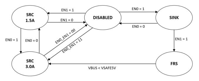
Figure 7. Sink and Source With FRS State Machine
