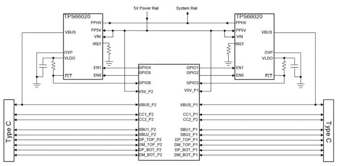
Figure 1. Typical Two Port System With TPS66020
