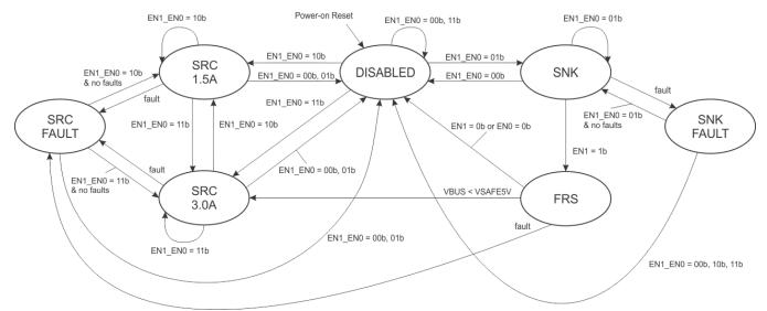
Figure 10. Sink and Source With FRS and Fault State Machine
