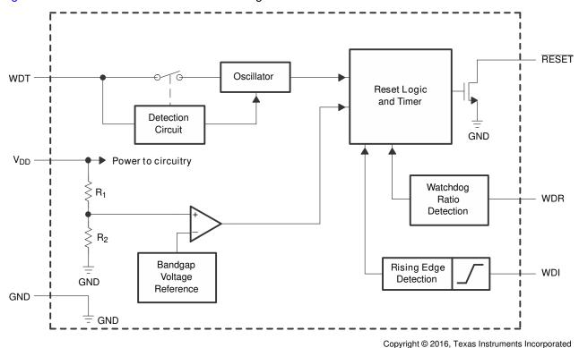
Figure 1-1. Functional Block Diagram
