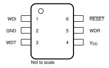
Figure 4-1. Top View 6-Pin SOT-23 DBV Package
