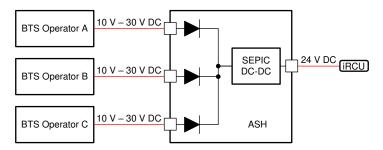
Figure 2-1. ORing Diodes Solution for ASH PowerPath Management
