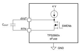
Figure 2-4. Output Slew Rate Control Set by CdVdT
