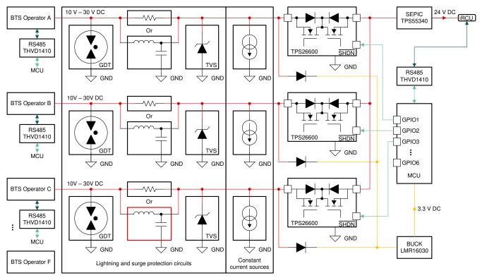
Figure 3-1. Typical ASH System Block Diagram Using TPS26600
