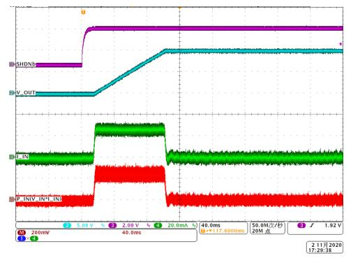
Figure 5-2. Start-up Inrush Current Control Waveforms at 10 V Input, without Load
