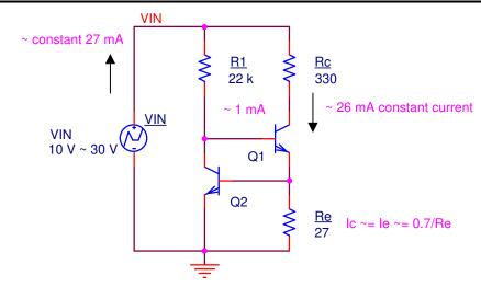
Figure 3-3. A Simple 27mA BJT Constant Current Source
