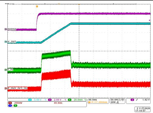
Figure 5-4. Start-up Inrush Current Control Waveforms at 10 V Input, 1Kohm Load
