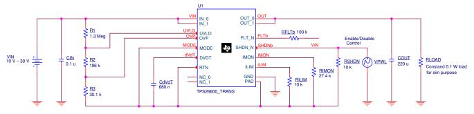
Figure 3-2. One Practical TPS26600 Circuit for ASH PowerPath Management
