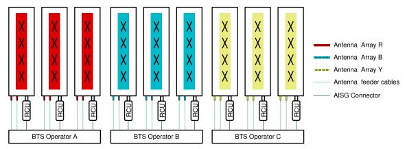
Figure 1-1. Single-band Antenna Deployment for Single Mode of Three Operators
