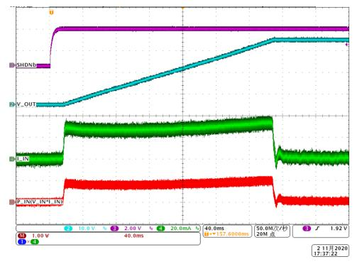
Figure 5-3. Start-up Inrush Current Control Waveforms at 30 V Input, without Load
