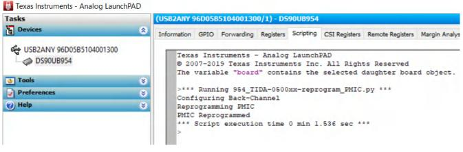
Figure 3-5. Analog LaunchPad Scripting Window
