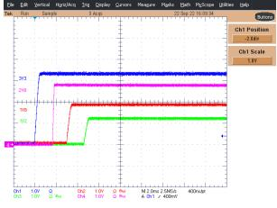
Figure 3-7. TPS65033000 Power Sequence After Reprogramming
