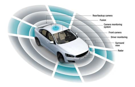
Figure 1-1. ADAS Camera Applications
