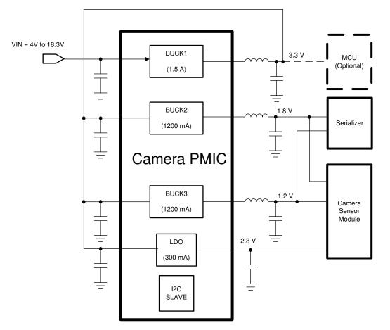
Figure 2-1. Typical Automotive Camera Application
