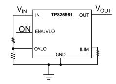
Figure 2. TPS25961 Configured for Programmable OVP and OCP
