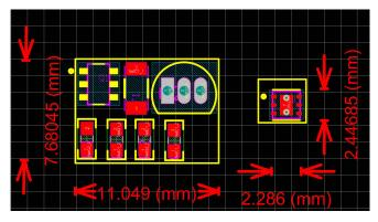
Figure 3. Discrete vs. TPS25961 Design Size
