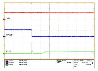
Figure 8. TPS25961 Short at Output Protection
