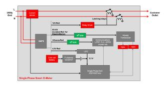
Figure 6. Single Phase Smart E-meter
