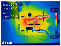
Figure 4-25. Thermal Condition in Single Phase Boost (V<sub>IN</sub>=10 V and 7 A Load)
