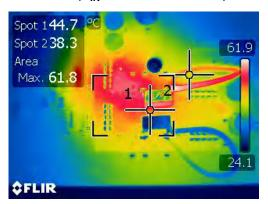
Figure 4-33. Thermal Condition in Single Phase Buck (V<sub>IN</sub>=24 V and 9 A Load)
