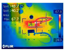
Figure 4-19. Thermal Condition in Single Phase Boost (V<sub>IN</sub>=8 V and 4 A Load)
