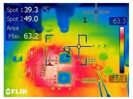
Figure 4-17. Thermal Condition in Buck Region (V<sub>IN</sub>=24 V and 8 A Load)
