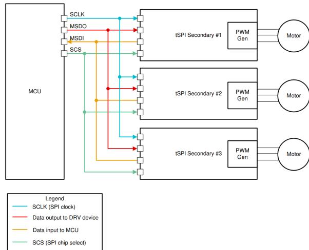
**Figure 1. Multi-Motor Control using tSPI**
