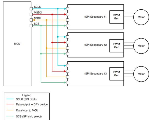
**Figure 1. Multi-Motor Control using tSPI**
