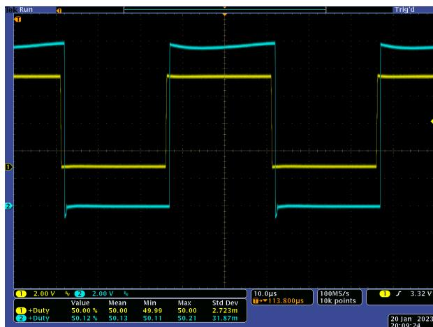
**Figure 4. DRV8311H Measured Duty Cycle at 50.0%**
