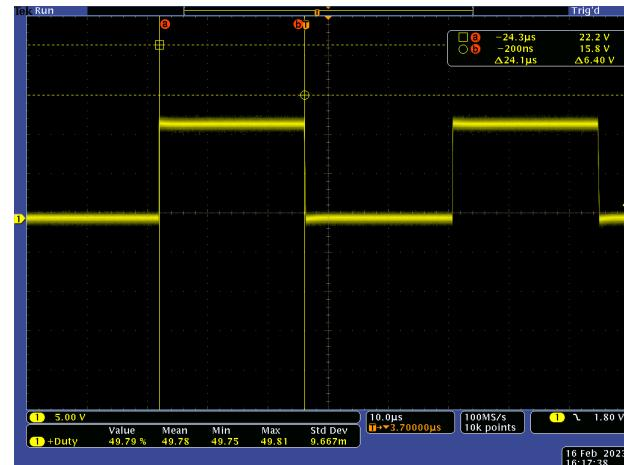
**Figure 2. DRV8311P Measured Duty Cycle at 50.0%**
