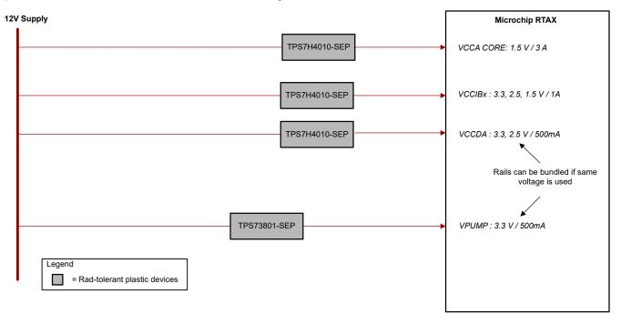
Figure 4-2. Rad-Tolerant Power for RTAX
