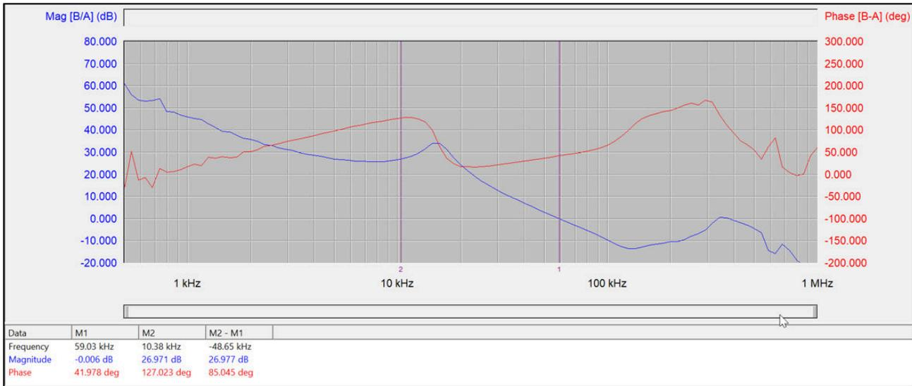
**Figure 5-1. Experimental Result With  $C2= 150\text{ }\mu\text{F}$ ,  $5\text{-m}\Omega$  ESR**
