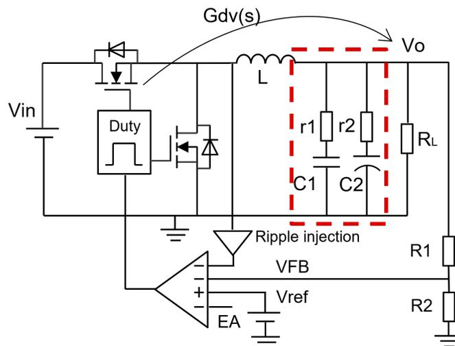
Figure 2-2. D-CAP3™ Functional Block Diagram With Hybrid Capacitor Network
