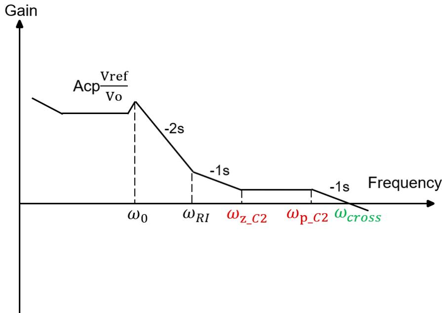
**Figure 4-2. Loop Gain of a D-CAP3™ Converter With  $\omega_{z\_C2} < \omega_{cross}$**
