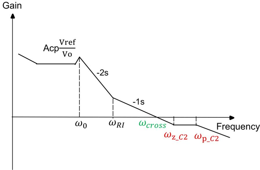
**Figure 4-1. Loop Gain of a D-CAP3 Converter With  $\omega_{z\_C2} > \omega_{cross}$**
