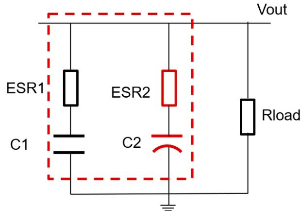
**Figure 2-1. The Simplified Equivalent Circuit of Hybrid Output Capacitors**
