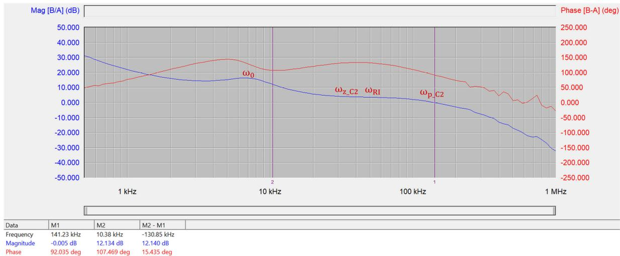
Figure 3-1. The Bode Plot Results of Bench Loop Test
