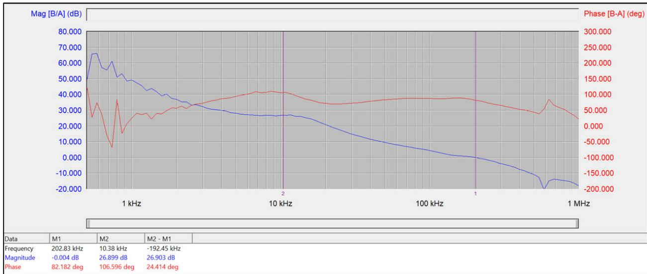
**Figure 5-2. Experimental Result With C2= 150  $\mu$ F, 70-m $\Omega$  ESR**
