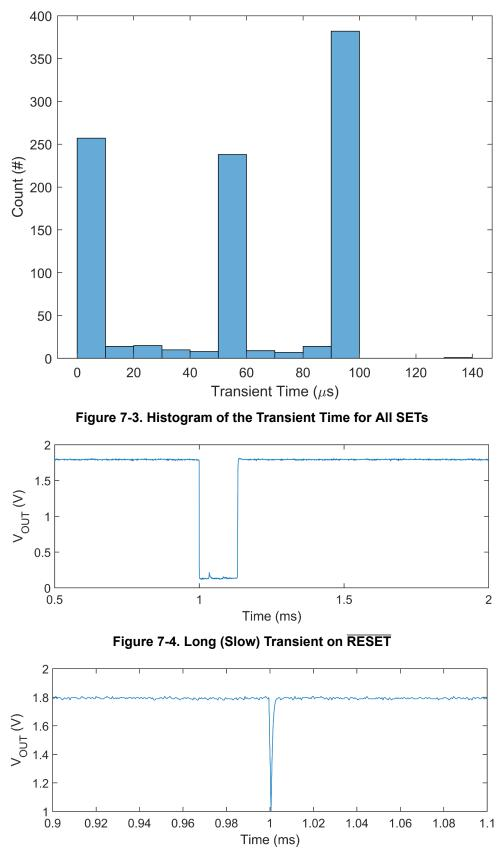
Figure 7-5. Short (Fast) Transient on RESET
