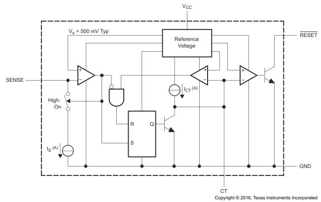
Figure 3-1. Functional Block Diagram of the TL7700-SEP
