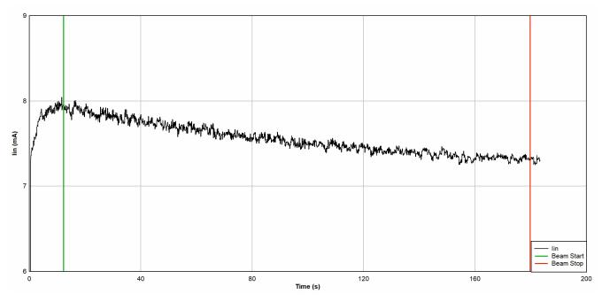
Figure 7-2. Current vs Time (I vs t) Data for V<sub>s</sub> Current During SEB Run #7
