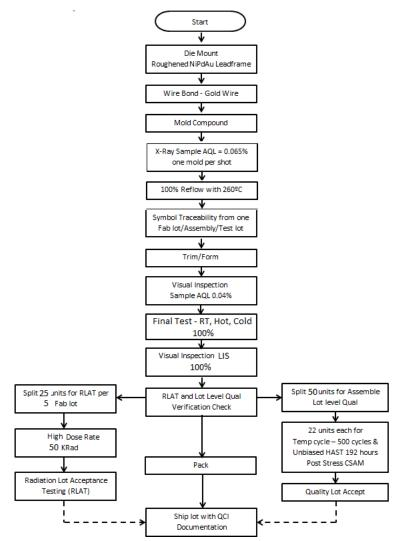
Figure 2-1. TPS7H4003-SEP Space Enhanced Plastic Production Flow Chart
