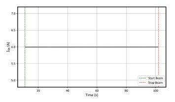
Figure 7-2. Current vs Time for Run # 4 (Enabled) for the TPS7H2201-SEP at T = 25°C
