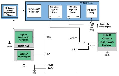
Figure 6-1. Block Diagram of SEE Test Setup With the TPS7H2201-SEP
