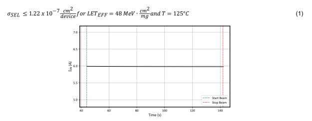
Figure 7-1. Current vs Time for Run # 1 of the TPS7H2201-SEP at T = 125°C
