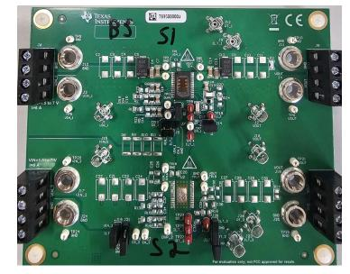
Figure 3-2. TPS7H2201-SEP Board Top View
