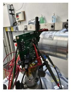
Figure 4-1. Photograph of the TPS7H2201-SEP Evaluation Board Mounted in Front of the Heavy-Ion Beam Exit Port at the Texas A&M Cyclotron
