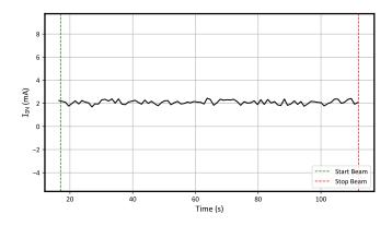
Figure 7-3. Current vs Time for Run # 5 (Disabled) for the TPS7H2201-SEP at T = 25°C
