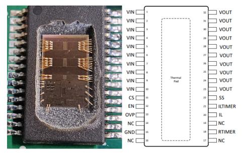
Figure 3-1. Photograph of Delidded TPS7H2201-SEP (Left) and Pin Out Diagram (Right)
