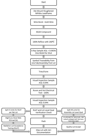
Figure 2-1. TPS7H2211-SEP Space Enhanced Plastic Production Flow Chart
