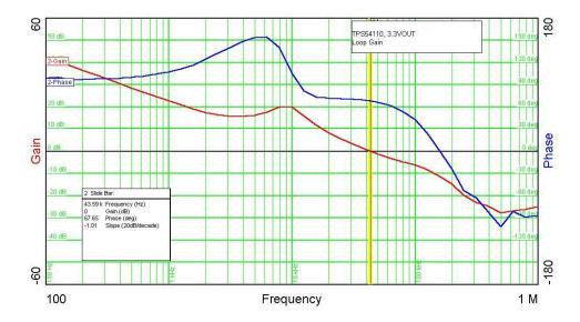
The figure below is the loop gain of the TPS54610 converter with max load. The bandwidth is 12 KHz, the phase margin is 59 degrees, and the gain margin is 28dB.
