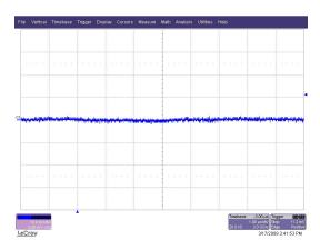
Output ripple/noise 1.2V output:
