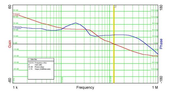
The figure below is the loop gain of the 1.2V converter with a 2.2A load. The bandwidth is 44.9 KHz, the phase margin is 56 degrees, and the gain margin is 22dB.
