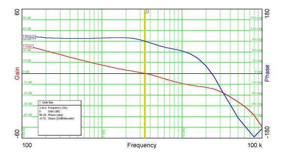
The figure below is the loop gain of the 2.5V converter with a 350mA load. The bandwidth is 113.8 KHz, the phase margin is 54 degrees, and the gain margin is 14dB. The 2.5V loop was measured with U6-4 (FB1) connected to TP7.
