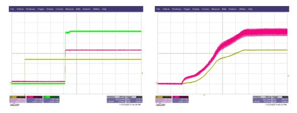
Output voltage turn-on response with a 48V input and a max load of 3.3V, 2.5V, 1.8V, and 1.2V showing sequencing :
