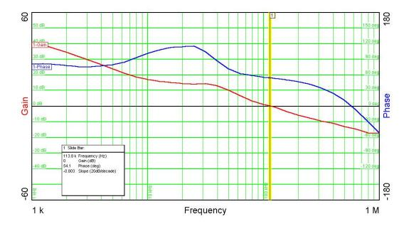
The figure below is the loop gain of the 1.8V converter with a 680mA load. The bandwidth is 122.6 KHz, the phase margin is 42 degrees, and the gain margin is 16dB.
