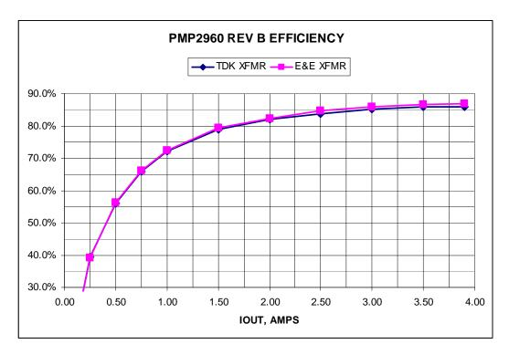
The end to end efficiency is: Outputs: 5.20V/15mA; 3.33V/2.00A; 2.49V/682mA; 1.80V/352mA; 1.20V/2.20A. Input: 48.0V/305mA Efficiency: 80.0%
