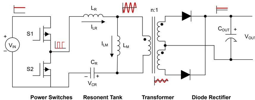
Figure 2. LLC Converter Example Block Diagram
