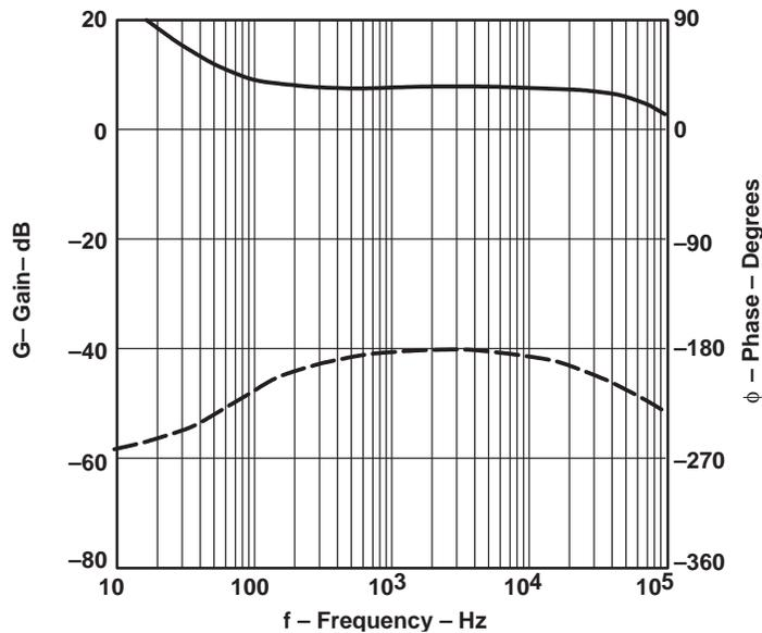
The overall open loop frequency response of the converter is the product of the uncompensated open loop response and the error amplifier response. A
