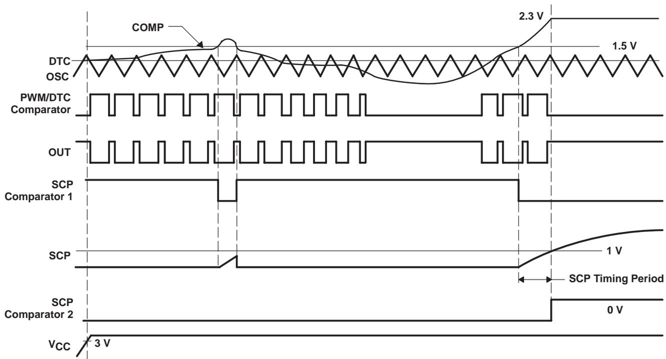
NOTE A: The waveforms show timing characteristics for an intermittent short circuit and a longer short circuit that is sufficient to activate SCP.
