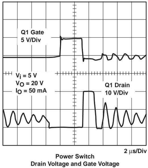
Figure 1–10. Pulse Load Response 50 mA to 100 mA
