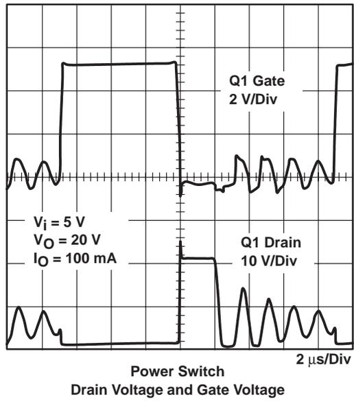
Figure 1–9. Power Switch Drain Voltage and Gate Voltage
