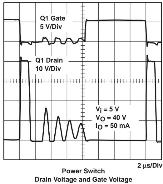
Figure 1–8. Power Switch Drain Voltage and Gate Voltage
