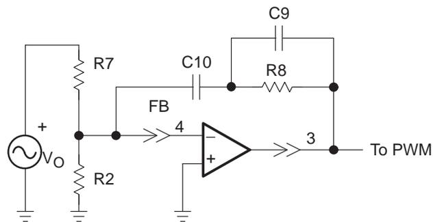
Assuming an ideal amplifier, the error amplifier transfer function is:
