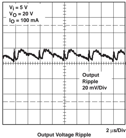
Figure 1–5. Output Voltage Ripple
