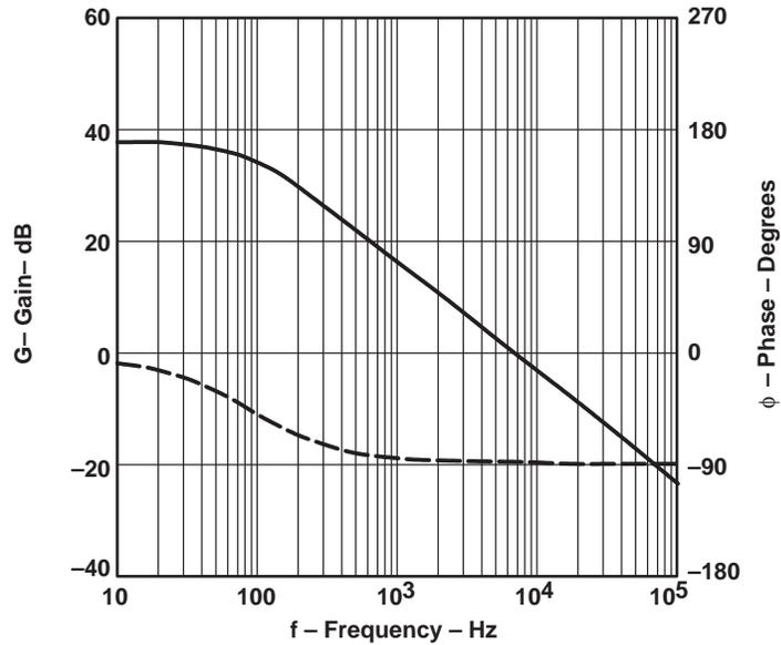
The presence of the single real pole is evident from the phase in the vicinity of 84 Hz and the fact that the total phase shift is only 90 degrees.
