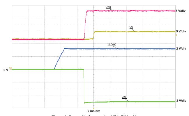
Figure 3. Power-Up Sequencing With EN2 =  $V_{IN}$
