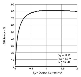
Figure 2. Buck Converter Efficiency
