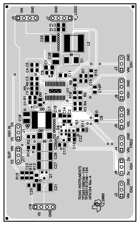
Figure 4. Top Assembly Layer
