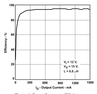
Figure 1. Boost Converter Efficiency
