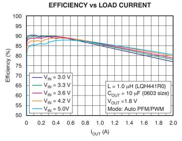
Figure 4. TPS62065, TPS62067 Efficiency vs Load Current
