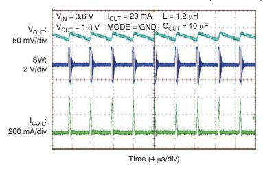
Figure 8. TPS62065 Output Voltage Ripple (PFM Mode)
