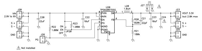
Figure 2. TPS62067EVM Schematic
