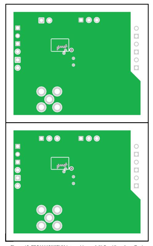
Figure 15. TPS62065/67EVM Internal Layer 2 (X-Ray View, from Top)
