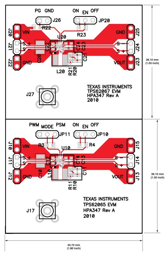
Figure 12. TPS62065/67EVM Component Placement (Top View)
