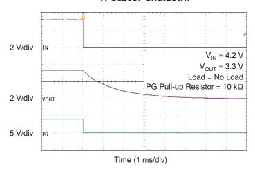
Figure 7. TPS62067 Shutdown: No Load
