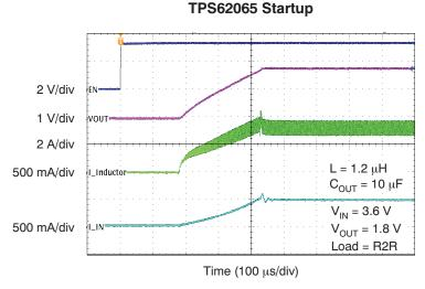
Figure 5. TPS62065 Startup into 2.2-Ω Load
