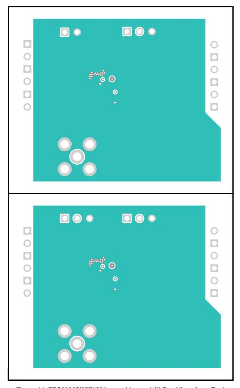
Figure 14. TPS62065/67EVM Internal Layer 1 (X-Ray View, from Top)
