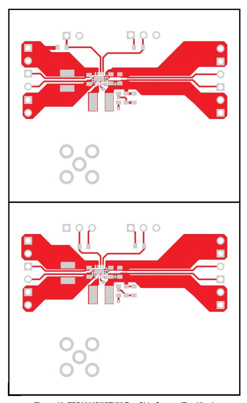
Figure 13. TPS62065/67EVM Top-Side Copper (Top View)
