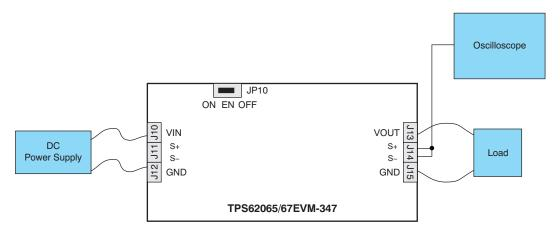
**Figure 3. Hardware Board Connection**
