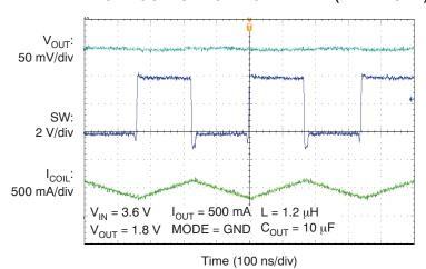
Figure 9. TPS62065 Output Voltage Ripple (PWM Mode)
