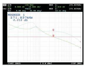
Conditions: VIN = 5.0 V, VOUT = 1.8 V,  $I_{OUT}$  = 1.6 A; bandwidth: 271 kHz, phase margin: 54°
