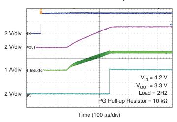
Figure 6. TPS62067 Startup into 2.2-Ω Load
