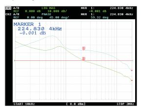
Conditions: VIN = 3.6 V, VOUT = 1.8 V,  $I_{OUT}$  = 1.6 A; bandwidth: 224 kHz, phase margin: 59°
