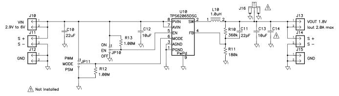
Figure 1. TPS62065EVM Schematic
