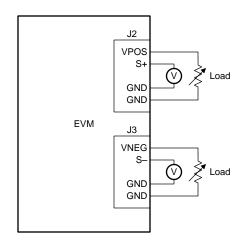
Figure 6. Single-Ended Load Connections
