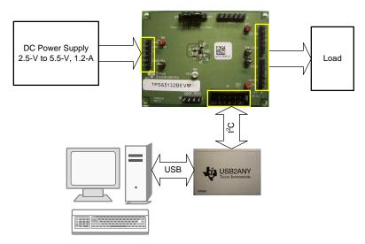
Figure 2. Hardware Setup – Full Functionality
