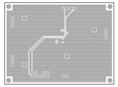
Figure 19. PCB Bottom Layer (Bottom View)
