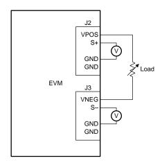
Figure 7. Differential Load Connection
