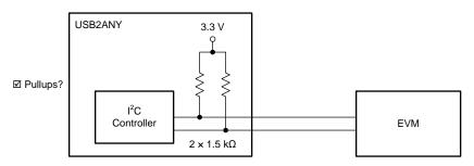
Figure 11. I<sup>2</sup>C Bus Internal Pullup Connection
