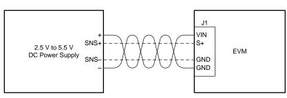
Figure 5. Four-Terminal Power Supply Connection
