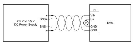
Figure 4. Two-Terminal Power Supply Connection
