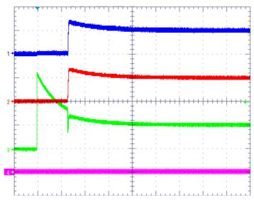
Figure 14. Input Surge (Not Clamped)
