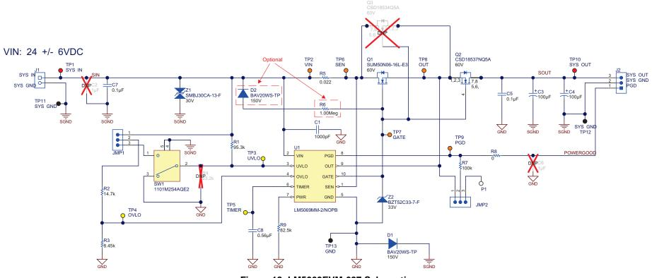
Figure 18. LM5069EVM-627 Schematic
