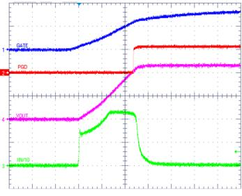
Figure 10. Turn-on Sequence with No Load Current
