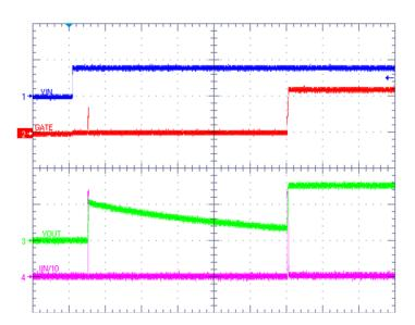
Figure 17. Inrush Current with 4900-µF Output Capacitor
