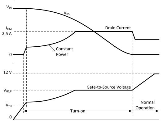
Figure 1. Power Up Using Power Limit and Current Limit
