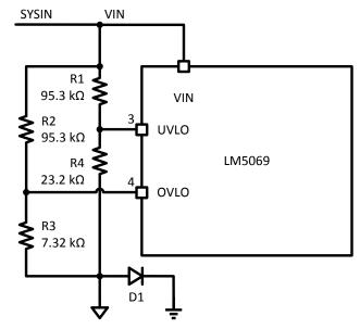
Figure 4. UVLO, OVLO Inputs (Option B)
