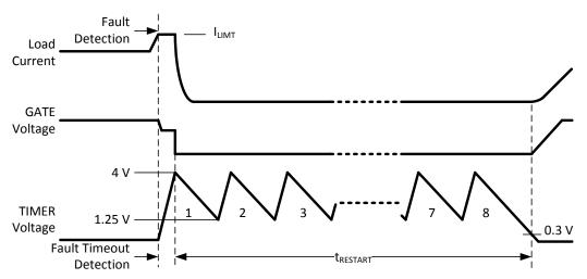
Figure 2. Fault Timeout and Restart Sequence
