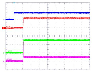
Figure 16. Inrush Current with 2550-µF Output Capacitor
