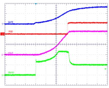
Figure 11. Turn-on Sequence with 1-A Load Current
