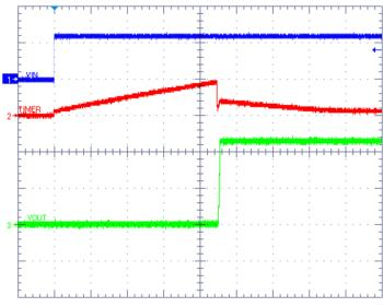
Figure 7. Insertion Timer Delay
