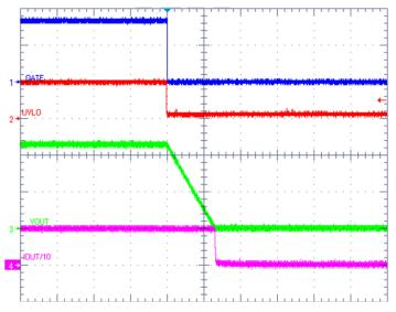
Figure 12. Output Shutdown Using UVLO Pin
