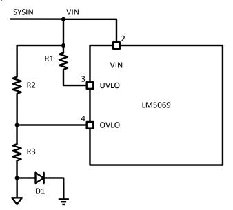
Figure 5. Minimum UVLO Threshold, Adjustable OVLO
