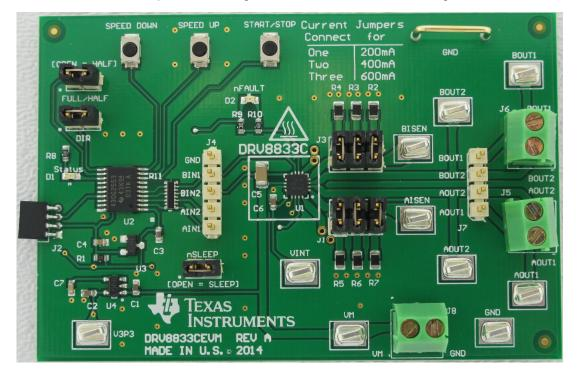
The motor connections are provided through connectors J5 and J6 on the right of the EVM.
