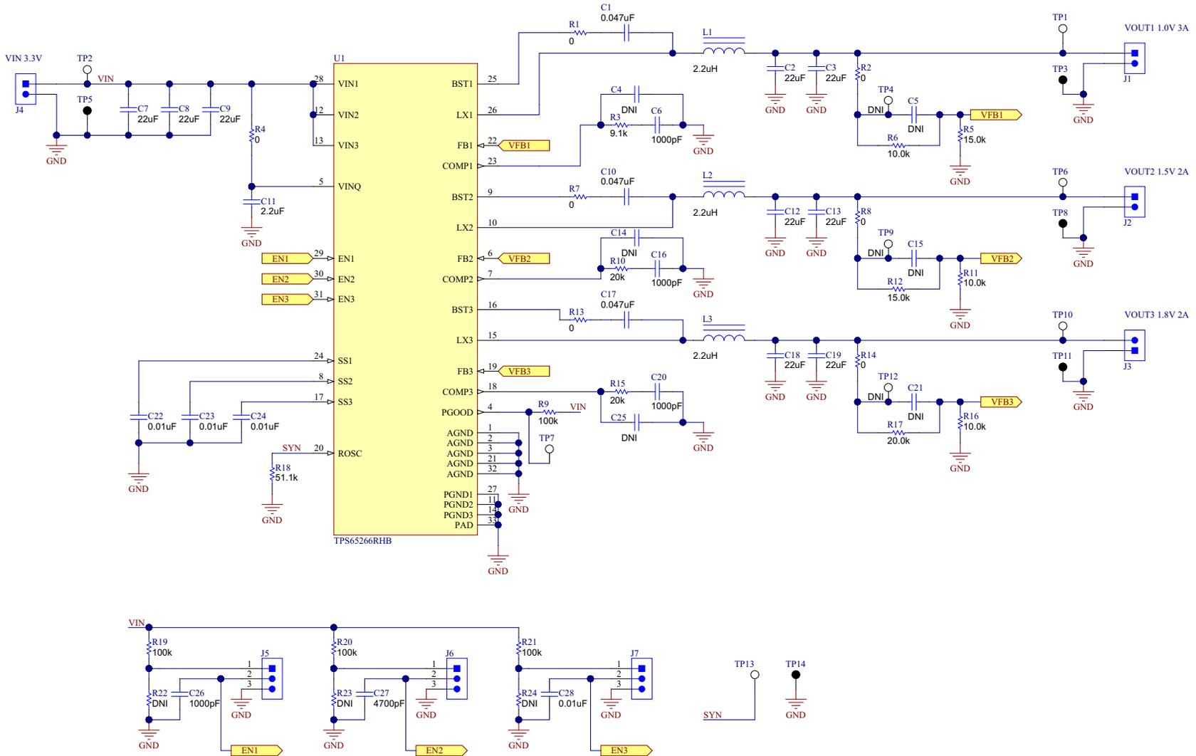
Figure 1. TPS65266EVM-686 Schematic
