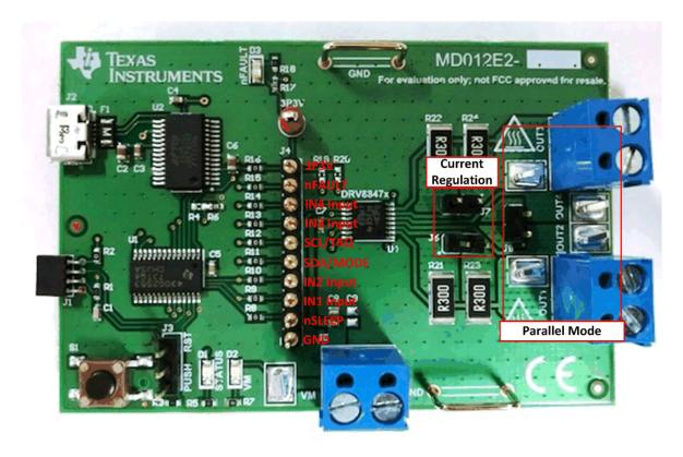
Figure 3. Test Points and Jumper Configuration
