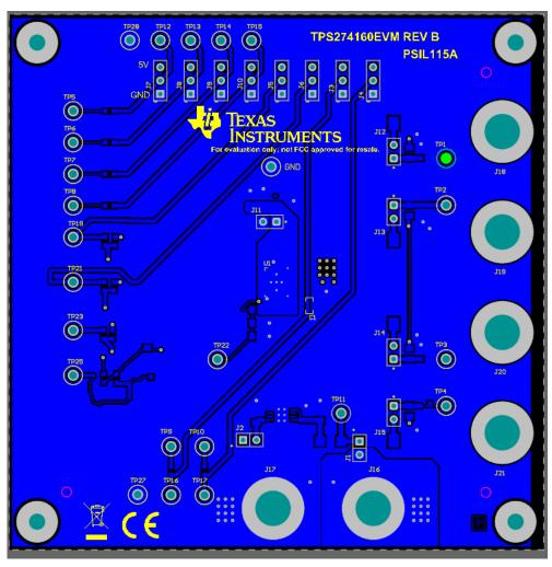
Figure 5. TPS274160EVM Bottom Layer (Top View)
