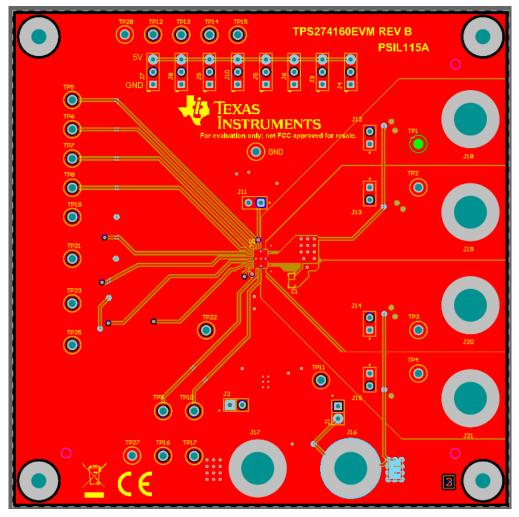
Figure 2. TPS274160EVM First Layer (Top View)
