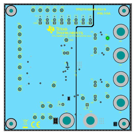
Figure 4. TPS274160EVM Third Layer Power Split (Top View)
