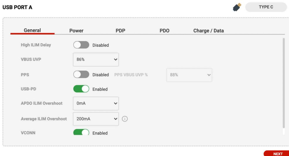
**Figure 4-1. USB Port Configuration Module**
