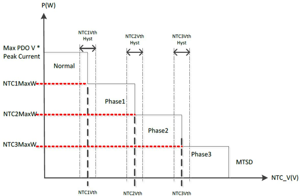
**Figure 4-3. Thermal Foldback Phase vs Maximum Port Power**
