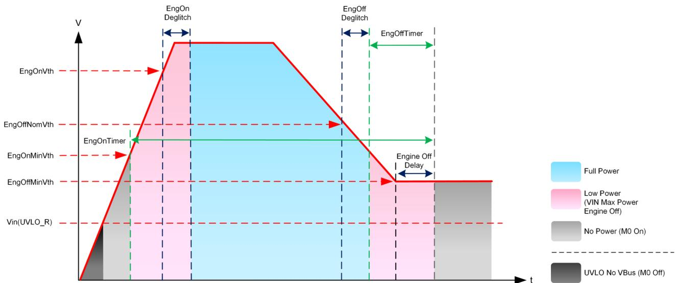
Figure 4-4. Engine On/Off Controls and Power Mode Operation
