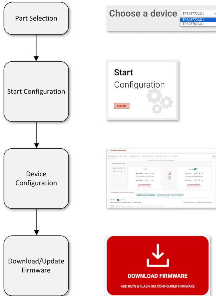
Figure 3-1. Typical GUI Flow
