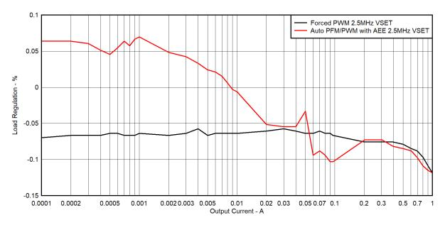
Figure 5-2. Load Regulation,  $V_{IN}$  = 6 V,  $V_{OUT}$  = 3.3 V,  $F_{SW}$  = 2.5 MHz
