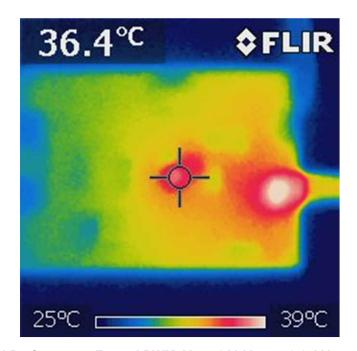
Figure 5-12. Thermal Performance Forced PWM,  $V_{IN}$  = 6 V,  $V_{OUT}$  = 3.3, V  $I_{OUT}$  = 1 A,  $F_{SW}$  = 2.5 MHz
