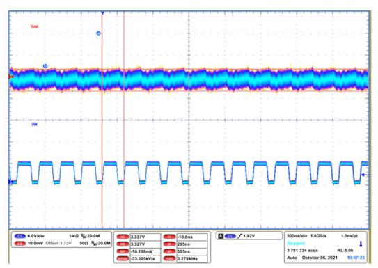
Figure 5-6. Output Voltage Ripple Forced PWM,  $V_{IN}$  = 6 V,  $V_{OUT}$  = 3.3 V,  $I_{OUT}$  = 1 A
