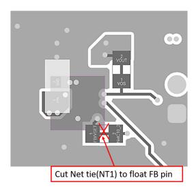
Figure 3-1. Internal Feedback (VSET) Configuration Board Modification
