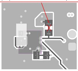
Figure 3-2. Bode Plot Measurement Board Modification
