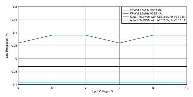
Figure 5-3. Line Regulation,  $V_{IN}$  = 5 V–10 V,  $V_{OUT}$  = 3.3 V,  $I_{OUT}$  = 0 A, and 1 A  $F_{SW}$  = 2.5 MHz
