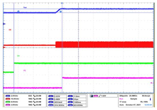
Figure 5-10. Enable Pre-Bias Start-Up Forced PWM,  $V_{IN}$  = 6 V,  $V_{OUT}$  = 3.3 V,  $I_{OUT}$  = 0 A
