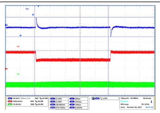
Figure 5-11. Load Transient Forced PWM VSET,  $V_{IN}$  = 6 V,  $V_{OUT}$  = 3.3 V,  $I_{OUT}$ = 0.5 A-1 A, Slew Rate = 1 A/us
