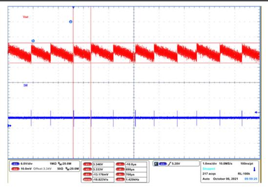
Figure 5-5. Output Voltage Ripple Auto PFM/PWM,  $V_{IN}$  = 6 V,  $V_{OUT}$  = 3.3 V,  $I_{OUT}$  = 0 A
