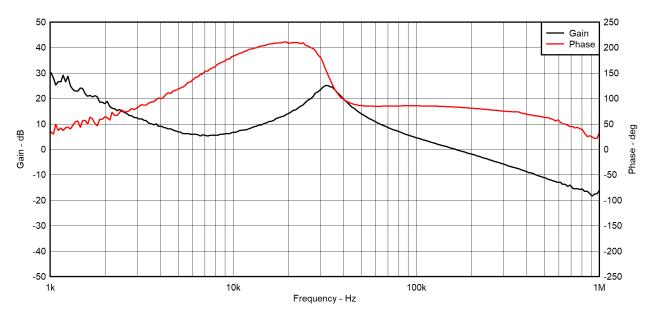
Figure 5-4. Loop Response Forced PWM VSET,  $V_{IN}$  = 6 V,  $V_{OUT}$  = 3.3 V,  $I_{OUT}$  = 1 A
