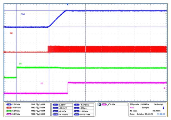
Figure 5-8. Enable Start Up Forced PWM,  $V_{IN}$  = 6 V,  $V_{OUT}$  = 3.3 V,  $I_{OUT}$  = 1 A
