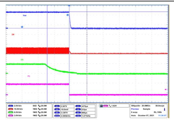
Figure 5-9. Enable Shutdown Forced PWM,  $V_{IN}$  = 6 V,  $V_{OUT}$  = 3.3 V,  $I_{OUT}$  = 1 A
