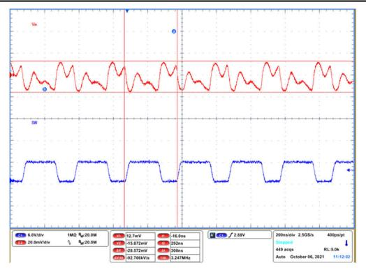
Figure 5-7. Input Voltage Ripple Forced PWM,  $V_{IN}$  = 6 V,  $V_{OUT}$  = 3.3 V,  $I_{OUT}$  = 1 A
