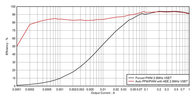
Figure 5-1. Efficiency,  $V_{IN}$  = 6 V,  $V_{OUT}$  = 3.3 V,  $F_{SW}$  = 2.5 MHz
