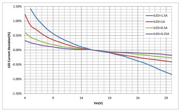
Figure 4-4. LED Current Deviation vs. Input Voltage in Analog Dimming Mode, 1 WLED
