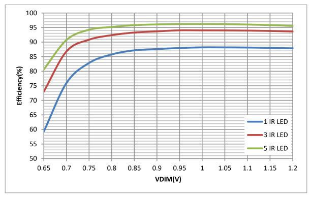
Figure 4-1. Efficiency vs. VDIM in Analog Dimming Mode(TPS92200D1RXLR), 1.5 A at VDIM>=1.2V,  $V_{IN} = 12 V$
