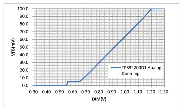
Figure 4-6. Output Current Ratio vs. VDIM in Analog Dimming Mode(TPS92200D1RXLR)
