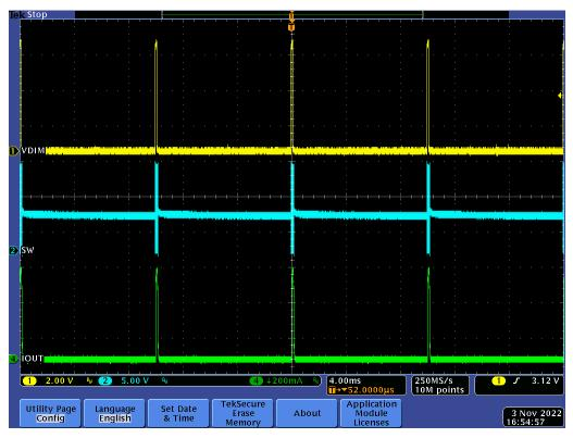
Figure 4-8. 1% Duty Cycle 100-Hz PWM Dimming(TPS92200D1RXLR)
