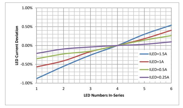
Figure 4-5. LED Current Deviation vs. LED Numbers in Series in Analog Dimming Mode, V<sub>IN</sub> = 24 V
