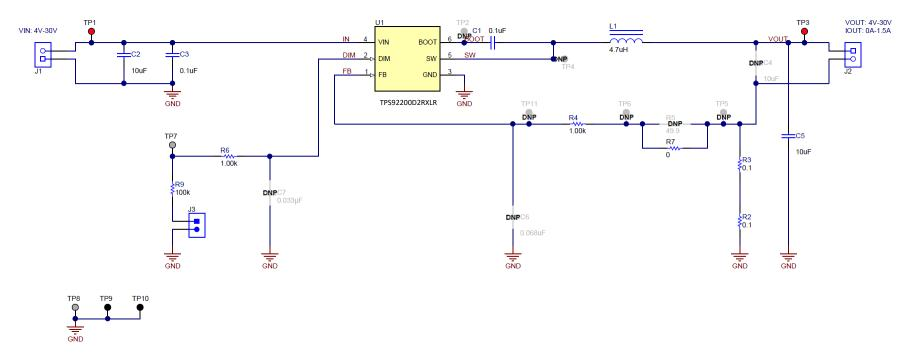
Figure 5-2. TPS92200D2RXLREVM Schematic
