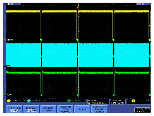
Figure 4-10. 95% Duty Cycle 100-Hz PWM Dimming(TPS92200D1RXLR)
