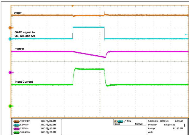
$V_{IN} = 12\text{ V}$ ,  $C_{TIMER} = 22\text{ nF}$ ,  $C_{OUT} = 470\text{ }\mu\text{F}$ ,  $R_{IMON} = 1.1\text{ }\parallel\text{ }1.1\text{ k}\Omega$ ,  $R_{REF} = 40.2\text{ k}\Omega$ ,  $I_{OUT}(\text{Steady-State}) = 100\text{ A}$ , and  $I_{OUT}(\text{Transient}) = 69\text{ A}$  for 9 ms
