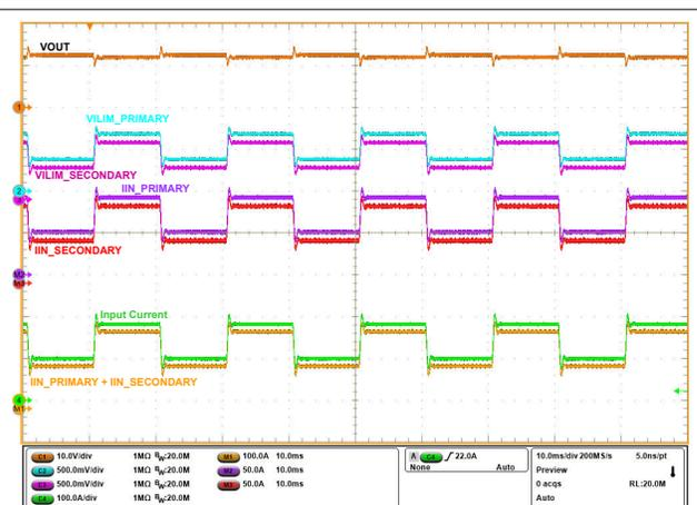
$V_{IN} = 12\text{ V}$ ,  $C_{TIMER} = 22\text{ nF}$ ,  $C_{OUT} = 470\text{ }\mu\text{F}$ ,  $R_{IMON} = 1.1\text{ }\parallel\text{ }1.1\text{ k}\Omega$ ,  $R_{IREF} = 40.2\text{ k}\Omega$ ,  $I_{OUT}$  ramped from 98 A to 180 A then 98 A within 10 ms
