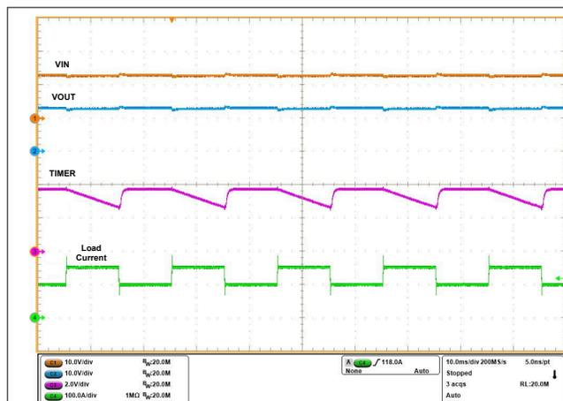
$V_{IN} = 12\text{ V}$ ,  $C_{TIMER} = 22\text{ nF}$ ,  $C_{OUT} = 470\text{ }\mu\text{F}$ ,  $R_{IMON} = 1.1\text{ }\parallel\text{ }1.1\text{ k}\Omega$ ,  $R_{IREF} = 40.2\text{ k}\Omega$ ,  $I_{OUT}$  ramped from 100 A to 175 A then 100 A within 10 ms
