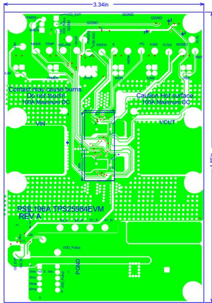
Figure 6-7. TPS25984EVM Board: Layer 4 (Signal)
