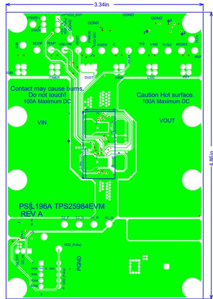
Figure 6-8. TPS25984EVM Board: Layer 5 (Signal)
