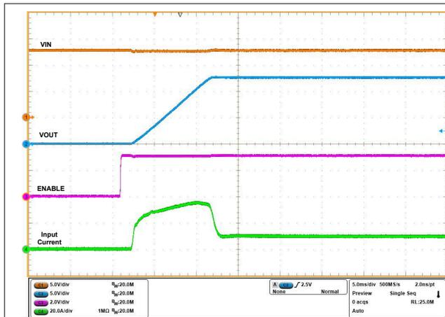
$V_{IN} = 12\text{ V}$ , EN stepped up from 0 V to 3 V,  $C_{OUT} = 18.47\text{ mF}$ ,
