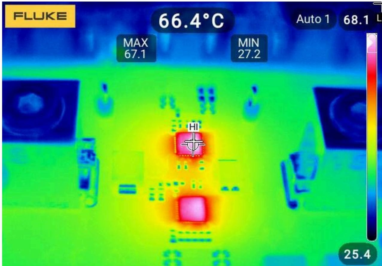
$V_{IN} = 12\text{ V}$ ,  $I_{OUT} = 110\text{ A}$ ,  $T_A = 25^\circ\text{C}$ , and no external air flow
