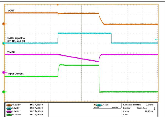
$V_{IN} = 12\text{ V}$ ,  $C_{TIMER} = 22\text{ nF}$ ,  $C_{OUT} = 470\text{ }\mu\text{F}$ ,  $R_{IMON} = 1.1\text{ }\parallel\text{ }1.1\text{ k}\Omega$ ,  $R_{REF} = 40.2\text{ k}\Omega$ ,  $I_{OUT}(\text{Steady-State}) = 100\text{ A}$ , and  $I_{OUT}(\text{Transient}) = 69\text{ A}$  for 18 ms
