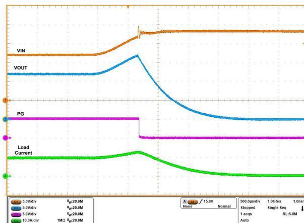
**Figure 5-10. Overvoltage Lockout Response of TPS25984 eFuse**
