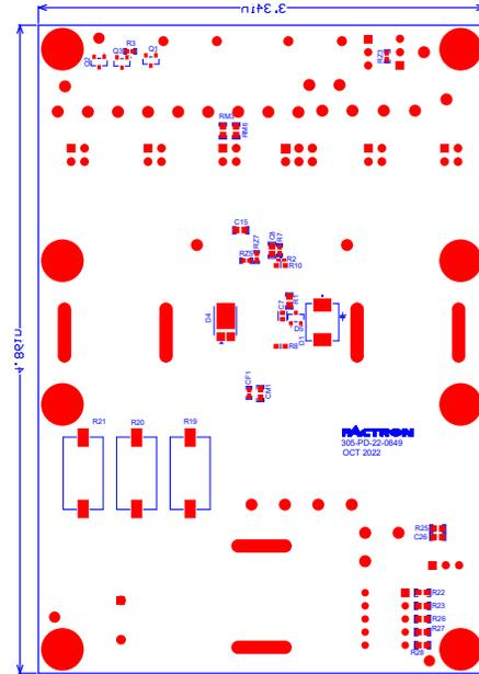
Figure 6-2. TPS25984EVM Board: Bottom Assembly
