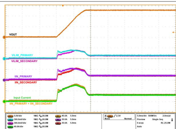
$V_{IN} = 12\text{ V}$ , EN stepped up from 0 V to 3 V,  $R_{LIM} = 400\text{ }\Omega$ ,
