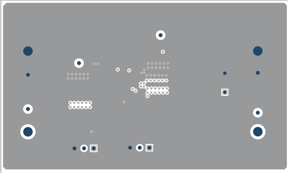
**Figure 3-4. Inner Layer 1 Layout**
