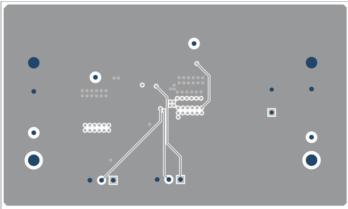
**Figure 3-5. Inner Layer 2 Layout**
