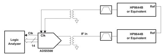
Figure 12. ADC Evaluation Test Set Up (Baseline)
