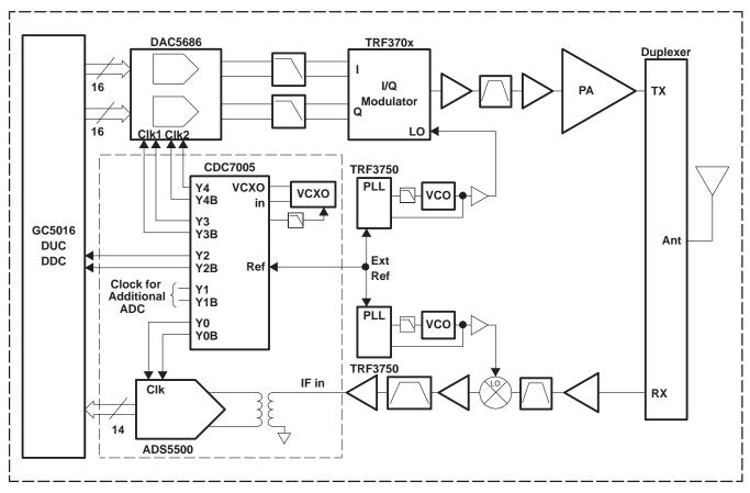
Figure 1. ADS5500 ADC With CDC7005 Clocking Solution Within A Typical Base Station Architecture
