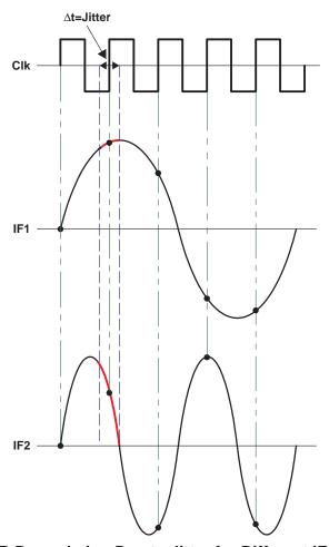
Figure 2. SNR Degradation Due to Jitter for Different IF Input Signals
