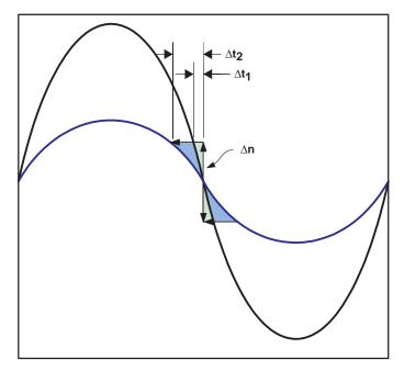
Figure 6. Thermal Noise Effect for Different Amplitude Sinusoids
