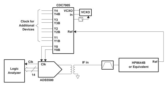
Figure 13. ADC Evaluation Test Setup With the CDC7005 Clocking Source
