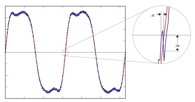
Figure 4. Thermal Noise Component Causing Sampling Error
