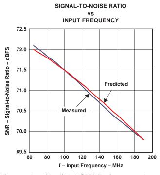
Figure 3. Measured vs Predicted SNR Performance Over Input Frequency
