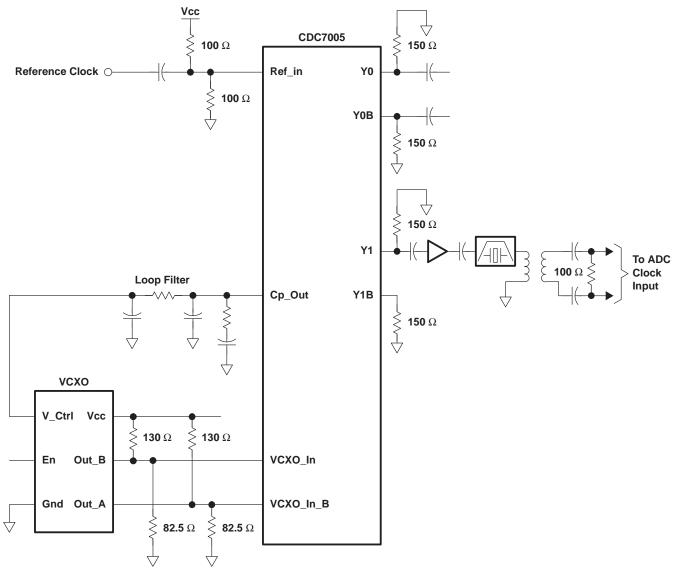
Figure 19. CDC7005 Clocking Topology With An Amplifier and Filter
