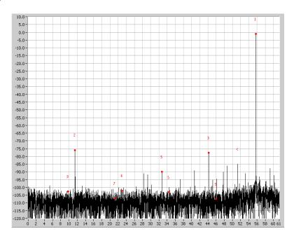
Figure 21. Spectral Plot With CDC7005 Clock Plus Amplifier-BPF at 190-MHz IF Input
