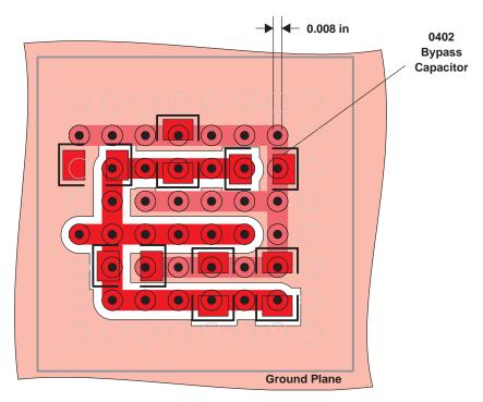
Figure 11. Supply Bypassing for the CDC7005
