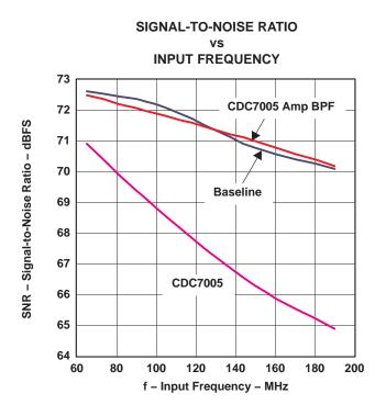
Figure 20. SNR Response With Improved Clocking Topology
