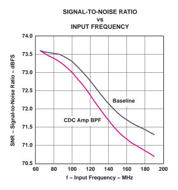
Figure 22. ADS5553 SNR Performance Over Input Frequency With New CDC7005 Clock Topology
