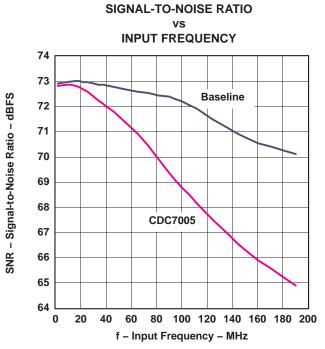
Figure 14. SNR Performance vs IF Input Frequency
