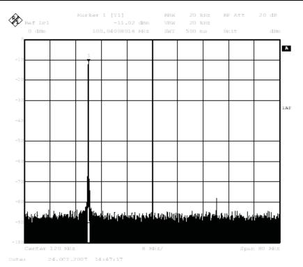
Figure 52. Filter Design Output Spectrum
