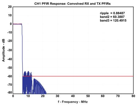
Figure 47. Complete Response of Successful Filter Design
