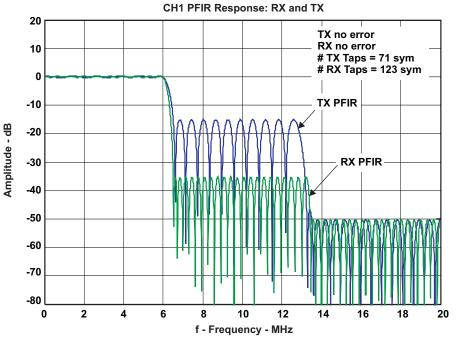
Figure 43. Redesigned Filter Response (without CIC Compensation)
