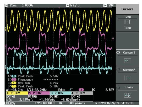
Figure 61. Incorrect Interface Timing for a Decimation of 6 and SCK Divider Ratio of 2
