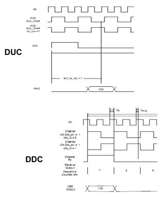
Figure 54. DUC Input Time
