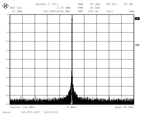
Figure 50. DAC Stand Alone Test Spectrum
