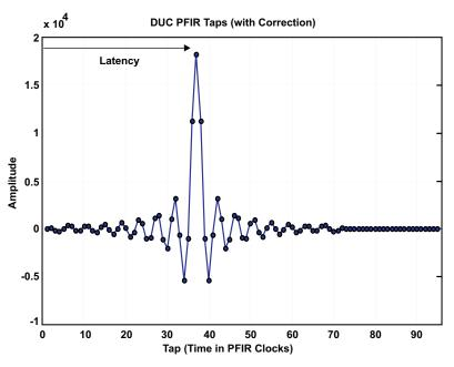
Figure 41. PFIR Tap and Filter Latency
