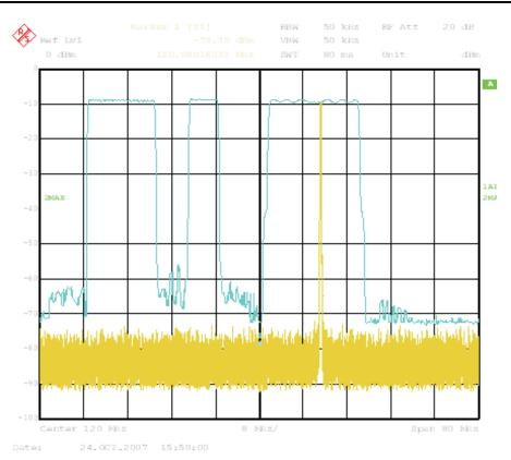
Figure 67. Multiple Channel Example on Spectrum Analyzer
