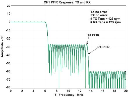
Figure 49. Filter with Reduced Stopband
