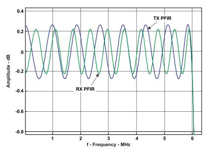
Figure 40. Magnified Filter Passband
