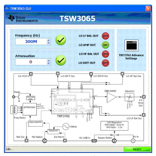
Figure 5. Screen shot of TSW3065EVM GUI
