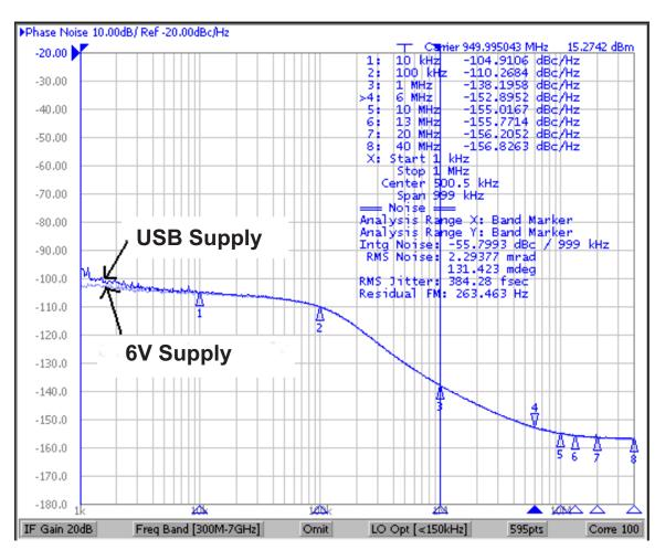
Figure 10. Phase Noise Comparison at 'LO Amp Out' at Maximum Output Power Using USB Supply and 6V Supply with Dip Switch at Position 0001–950MHz
