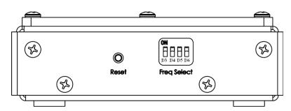
Figure 4. Dip Switch and Push Button
