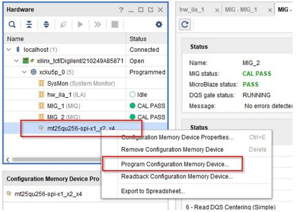
Figure 3-2. Programming Memory Device
