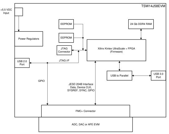
Figure 2-2. TSW14J58EVM Block Diagram
