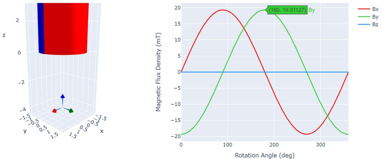
**Figure 3-7. Magnetic Field Strength Results at 4.0 mm with 1/8 Inch Magnet**
