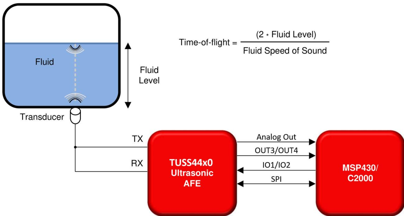
Figure 2-2. Ultrasonic Liquid Level Sensing
