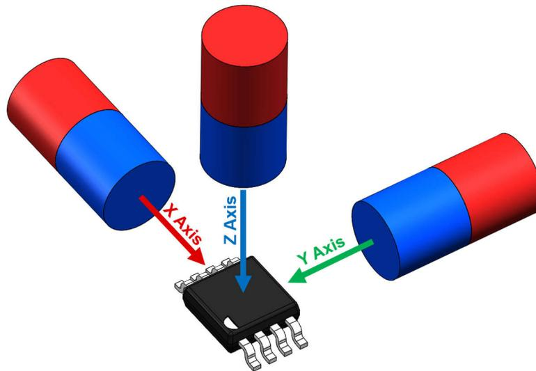
**Figure 2-3. 3D Hall Sensor Axis**
