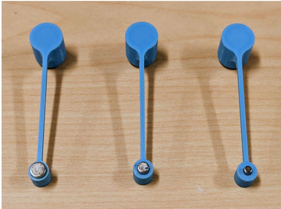
**Figure 3-6. Three Magnet Sizes in Float Arms**
