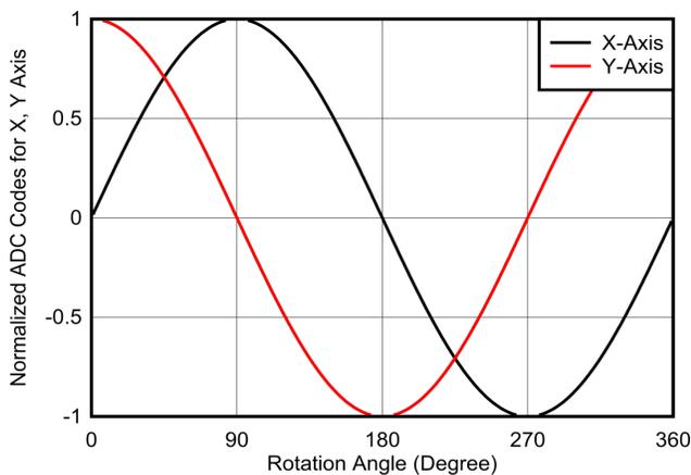
**Figure 2-10. X and Y Sensor Data for Full 360 Degree Rotation for On-Axis Measurement**
