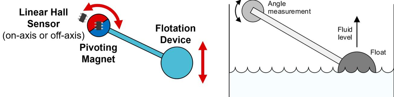
Figure 2-8. Pivoting Magnet Float Arm Implementation
