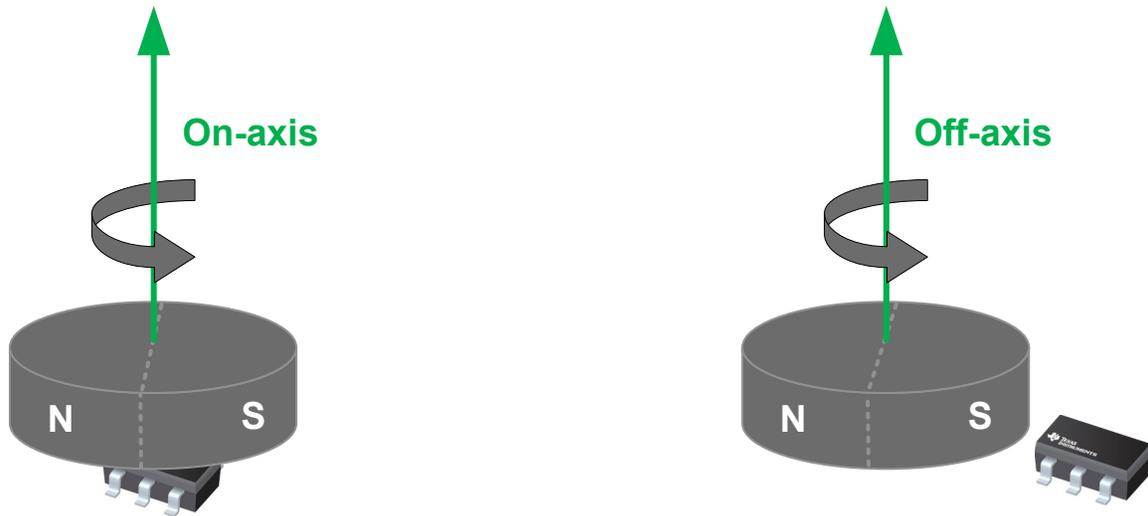
**Figure 2-9. On-Axis vs. Off-Axis Angle Measurements**
