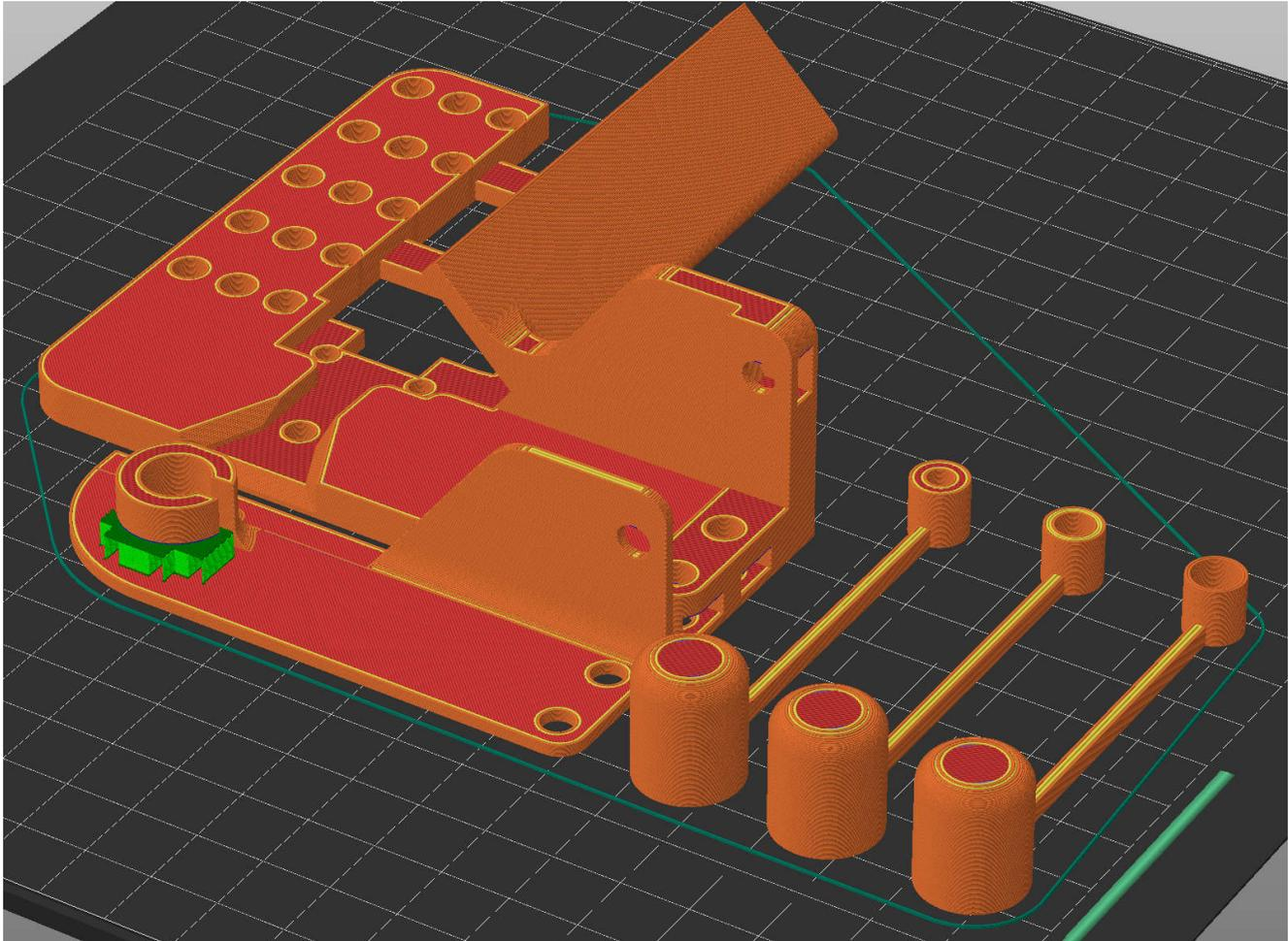
**Figure 3-12. Part Orientation in Slicer**
