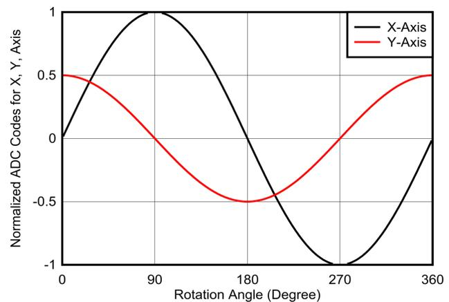
**Figure 2-11. X and Y Sensor Data for Full 360 Degree Rotation for Off-axis Measurement**
