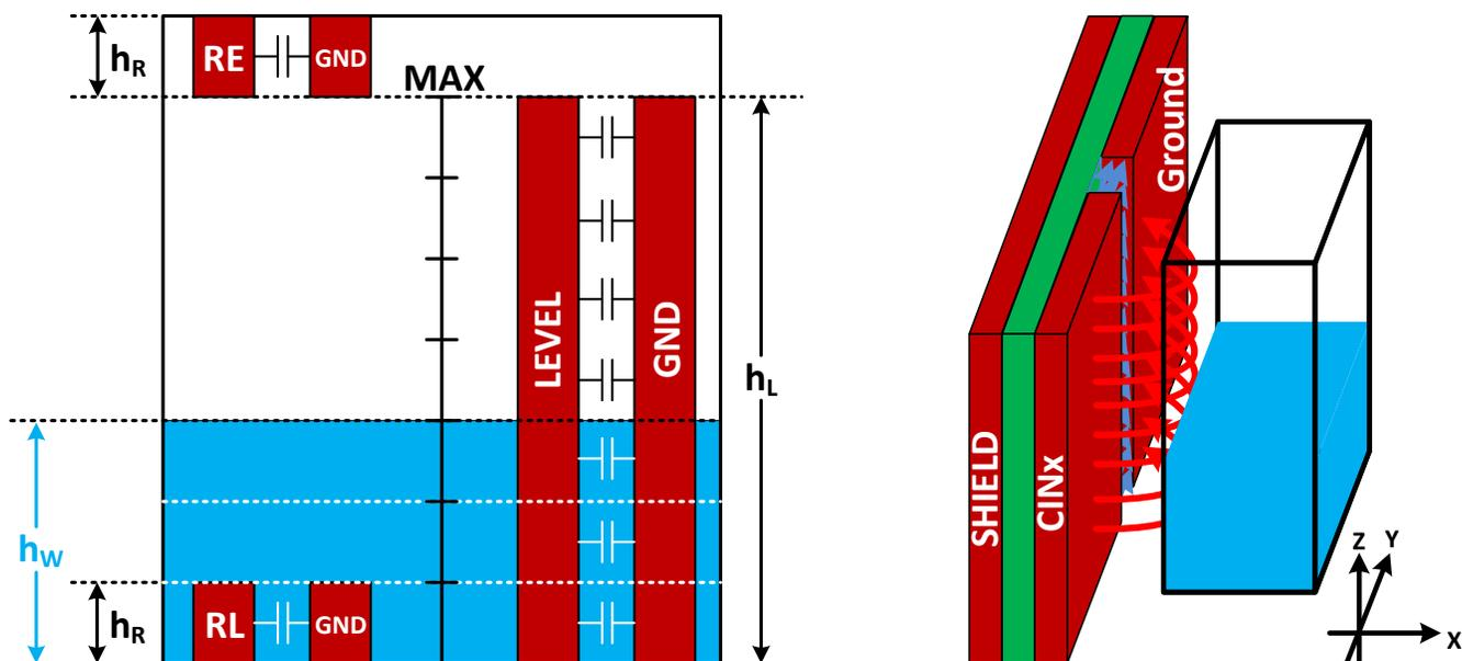
Figure 2-1. Capacitive Liquid Level Sensing
