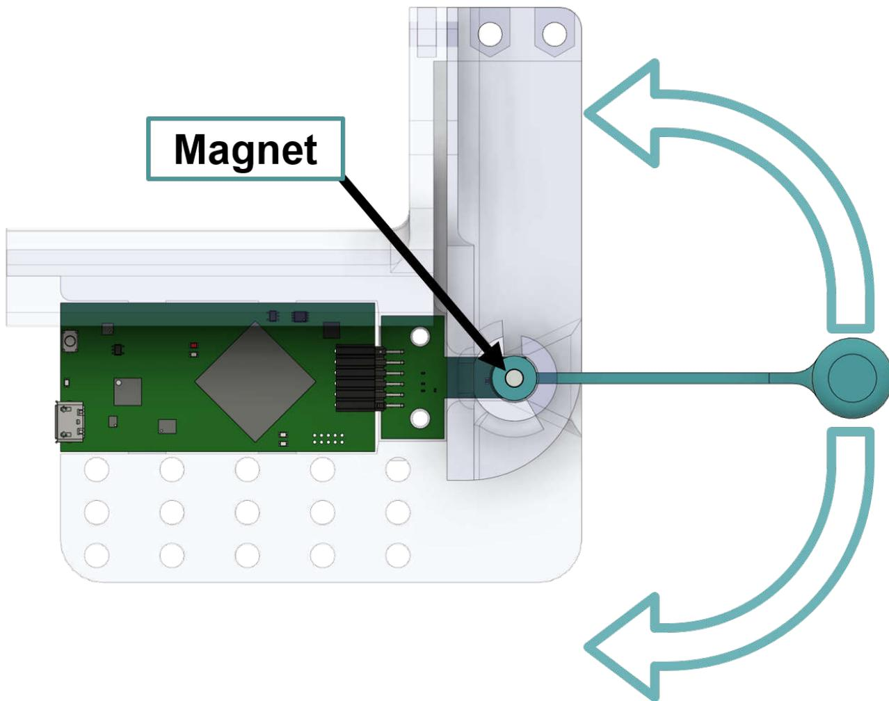
**Figure 3-5. Float Rotation and Magnet Placement**
