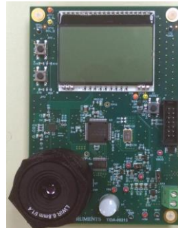
Thermopile-based occupancy sensing with an 8x8 array enabling people counting applications
