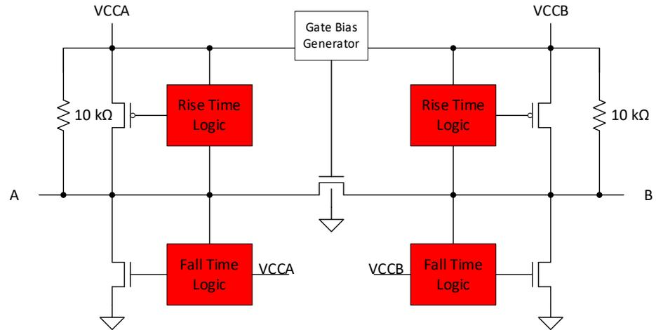
**Example of Rise Time & Fall Time Accelerator Circuit**
