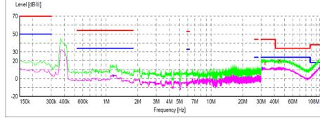
TPS25850 2.1 MHz EMI: CISPR25 CLASS5 PASS https://www.ti.com/tool/PMP40723
