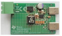
EMI standard : CISPR 25 Class5 PMP40723 FSW = 2.2MHz PASS PMP40680 FSW = 400kHz PASS
