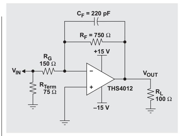
Figure 9. Inverting gain of 5 CFB configuration
