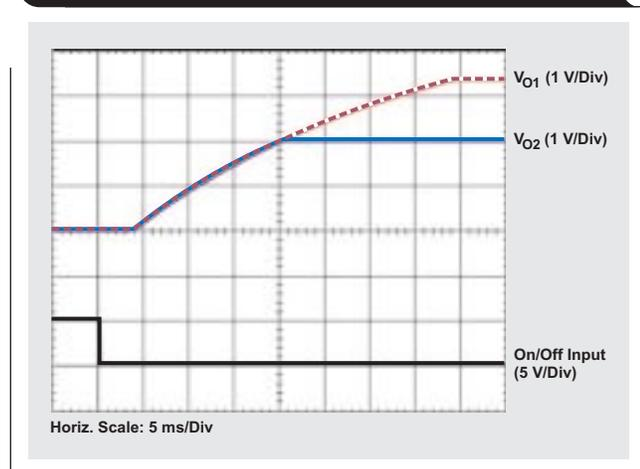
**Figure 4. Simultaneous power-down of two modules under Auto-Track Sequencing control**
