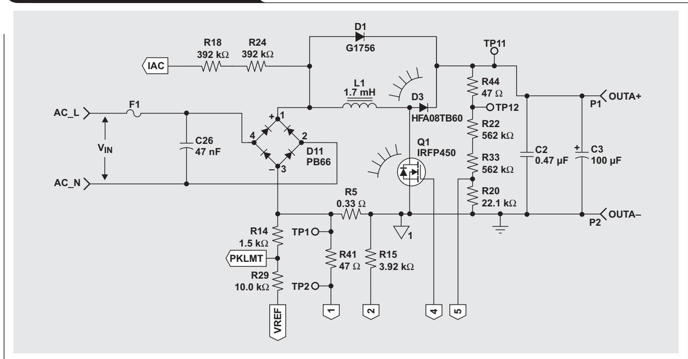
Figure 2. dc/dc power stage schematic
