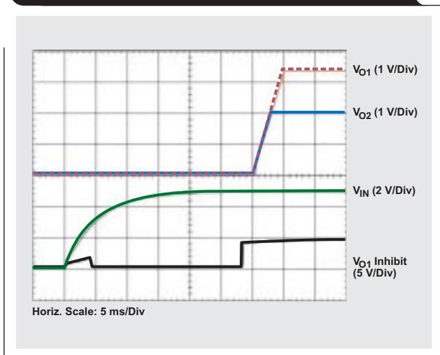
To initiate the power-up sequence, the U1 Inhibit control must be held to ground as input power is applied, then held there for another 20 ms. This allows time for the auto-tracking module, U2 (PTH05010W), to complete its internal power-up. In this circuit the TPS3838K33, a nanowatt supervisor IC (U3), is used both to detect the input voltage and to provide the required 20-ms time delay.
