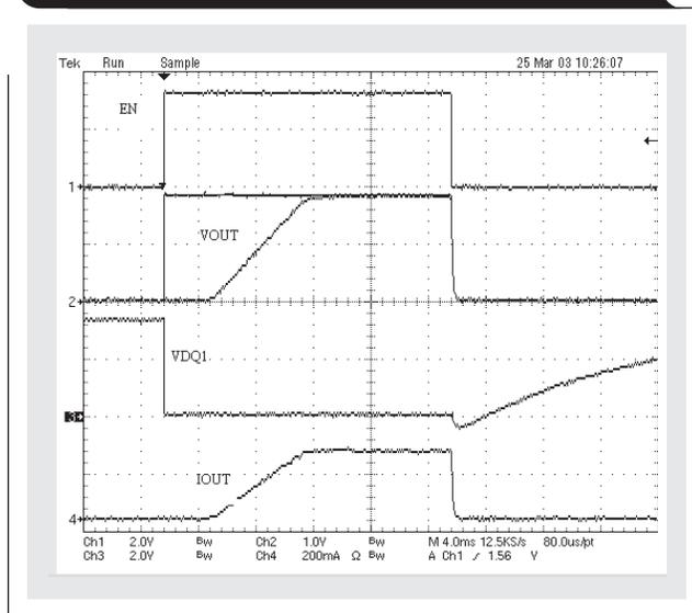
and thus could increase the lower tolerance limit of the regulator solution from  $-3$  to  $-3.8\%$ . In addition, to prevent large load transients from momentarily turning off the switch and causing the rail voltage to droop, a large output capacitor after the switch is recommended.
