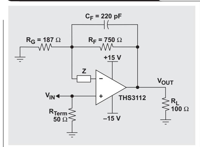
amplifier, can now be essentially any resistance desired. The reader should keep in mind that this is still a high-speed amplifier with speeds over 100 MHz; so the feedback resistance should always be kept less than a few kilohms to minimize the effects of parasitic capacitances on the overall circuit. Conversely, minimizing the resistance too much will place too much of a load on the amplifier, typically degrading performance.
