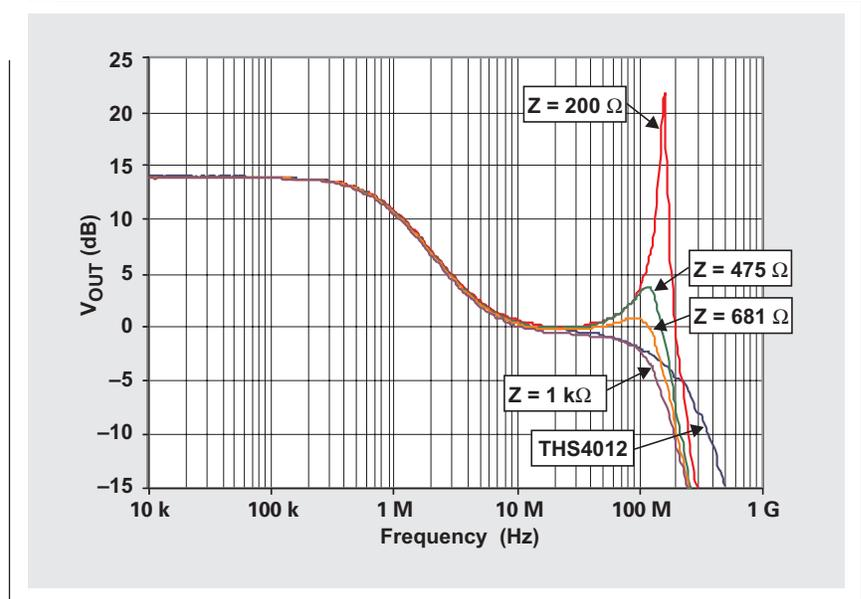
stated previously. This shows that there is a reasonably wide range of acceptable values for  $Z$  and does not imply that the selection for  $Z$  is highly critical. Figure 3 also illustrates a common trait for current-feedback amplifiers—as the feedback impedance is decreased, the peaking will increase. If the impedance is too low, there is a good chance that the circuit will become unstable and oscillate, as illustrated by the response when  $Z = 200 \Omega$ .
