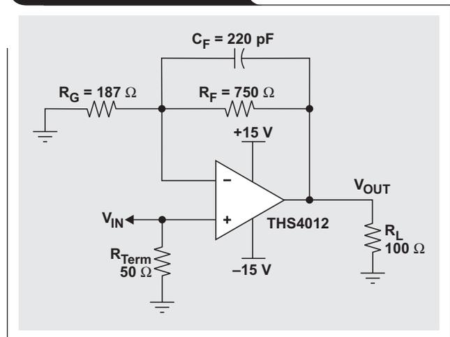
Figure 2. CFB test circuit with simple modification
