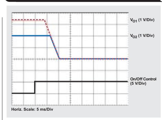
**Figure 5. Sequenced power-up and power-down with other modules**
