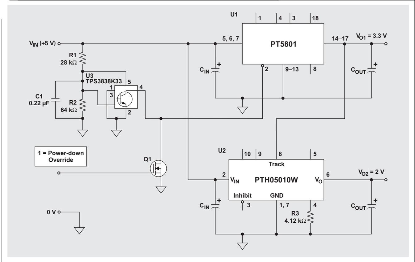
Figure 5 illustrates this arrangement. The Track pins of the lower-voltage modules must be connected directly to the output of the module with the *highest* output voltage, which in this case is PT5801 (U1). In this configuration, U1 must be controlled from its on/off Inhibit control pin.
