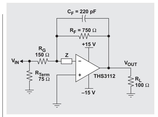
exactly the same as before. Figures 8 and 9 show the test circuits for this configuration. The signal gain was kept at a gain of 5.
