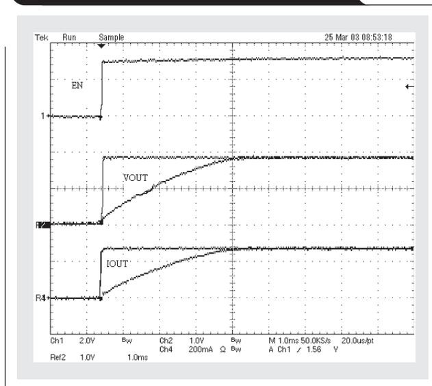
Either method limits the in-rush current, slowing the ramp time of the regulator output. The first method is best suited for higher-voltage rails with looser output-voltage tolerances and fewer transients. The second method provides the best performance, since the additional circuitry is effectively removed after startup and thus does not affect regulation; however, it will not work with all regulators.
