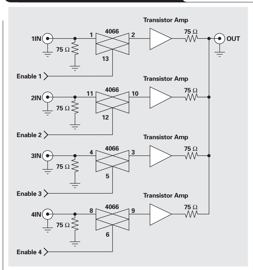
gain of 2 in the noninverting configuration, which compensates for a 75- $\Omega$  back termination resistor on the op amp output. Overall stage gain is therefore 1.
