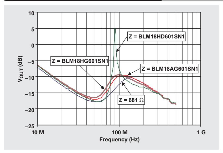
**Figure 12. Frequency responses with AG series ferrite chips (gain = -5)**
