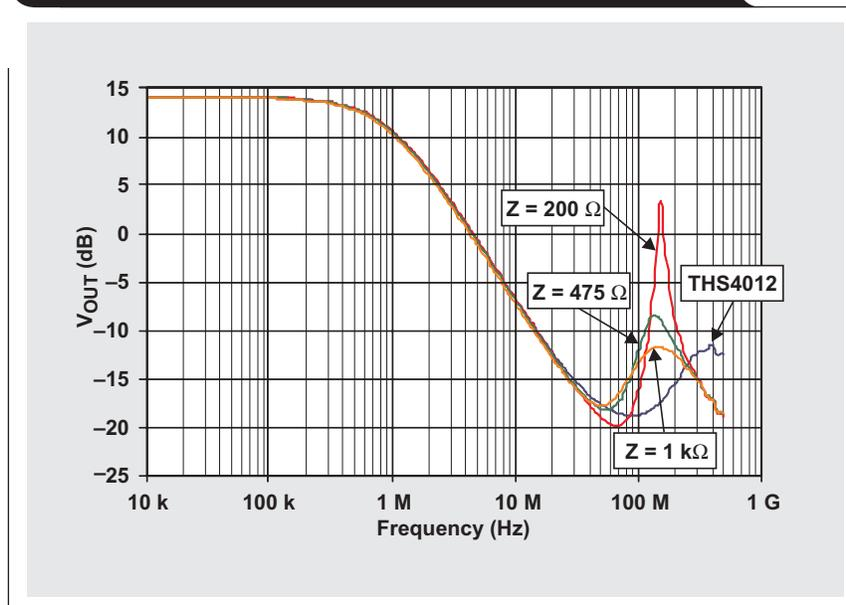
Figure 11 shows the frequency responses of several of these chips. Figure 12 shows the results of using various ferrite chips from the same AG family.
