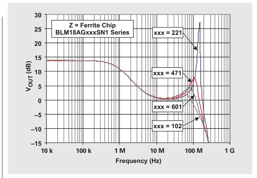
Figure 7. Output noise comparison (gain = +5)
