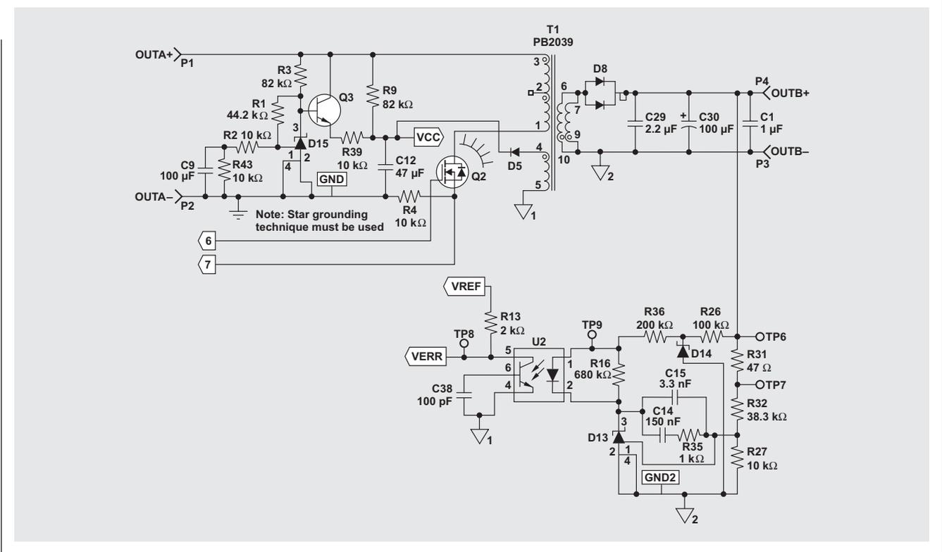
Figure 3. Controller schematic
