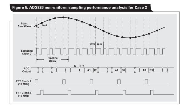
Figure 6. ADS826 non-uniform sampling performance analysis for Case 3
