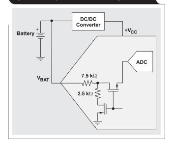
Figure 4. Using AUX with external voltage divider to monitor battery voltage
