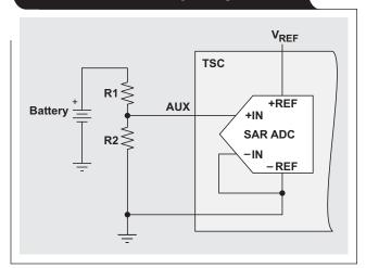
since the battery's voltage is normally higher than that of the TSC's power supply (and thus that of the  $V_{\rm REF}$ ).
