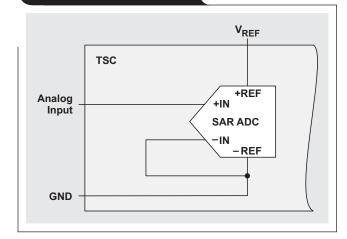
A TSC in differential mode does not need any reference, since the signal's driver is connected to +REF and –REF directly. However, the reference voltage,  $V_{\rm REF}$ , is a must for SE operation and thus is always needed when an auxiliary input, such as the AUX or  $V_{\rm BAT}$ , is measured.
