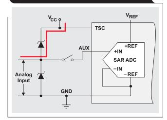
the analog input signal is active (AUX is nonzero) when the TSC is powered down ( $V_{\rm CC}=0$ ), the analog signal may be routed to the  $V_{\rm CC}$  through the ESD-protection diode (see the red line in Figure 6). This may partially or fully power up the TSC, depending upon the amplitude of the input signal, consuming more power and possibly causing the TSC to malfunction. Thus the circuit configuration in Figure 6 should be avoided.
