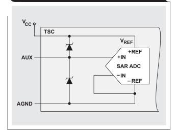
Some of TI's new TSCs, including the TSC2004/5/6/7, were designed with the enhanced, on-chip ESD protection shown by the simplified circuit in Figure 8. Obviously, for these devices, the input signal to the TSC's AUX should be removed before the TSC's  $V_{\rm CC}$  power is shut down. An example of removing the AUX signal is shown in Figure 9.
