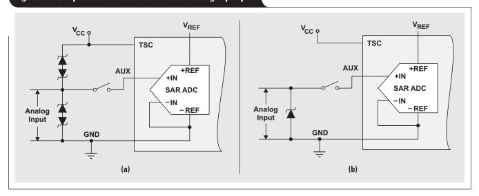
Figure 8. TSC2004/5/6/7 internal ESD protection for AUX input
