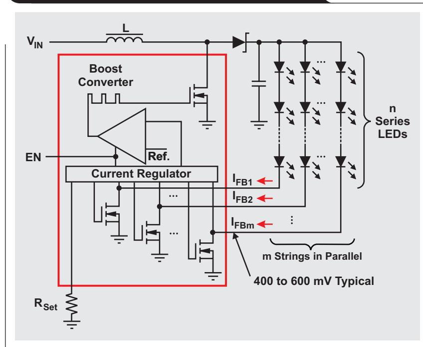
Figure 2 shows a driver with integrated current sinks. The driver samples the voltage at each current sink and ensures that the converter provides just enough power to keep the current sinks operational.
