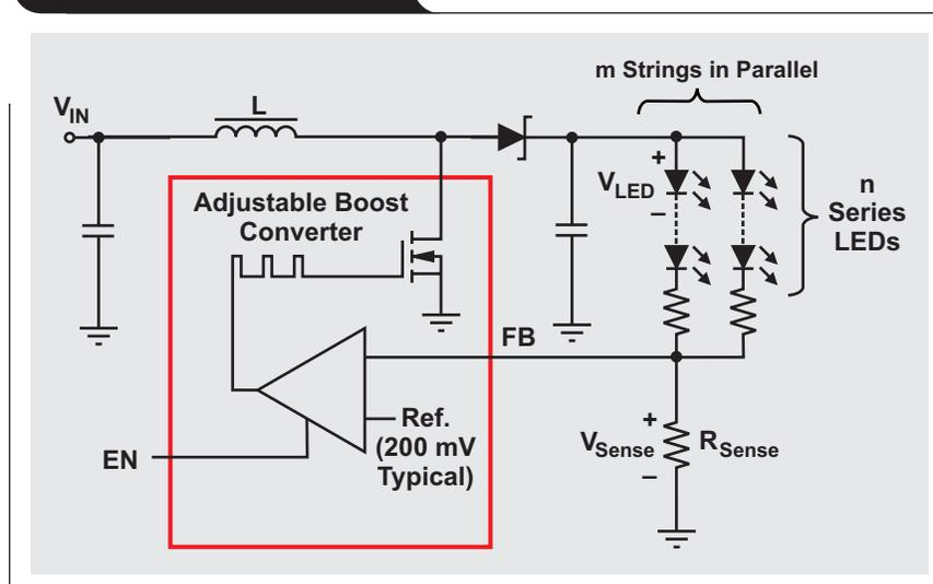
Figure 2. LED driver with integrated current sinks
