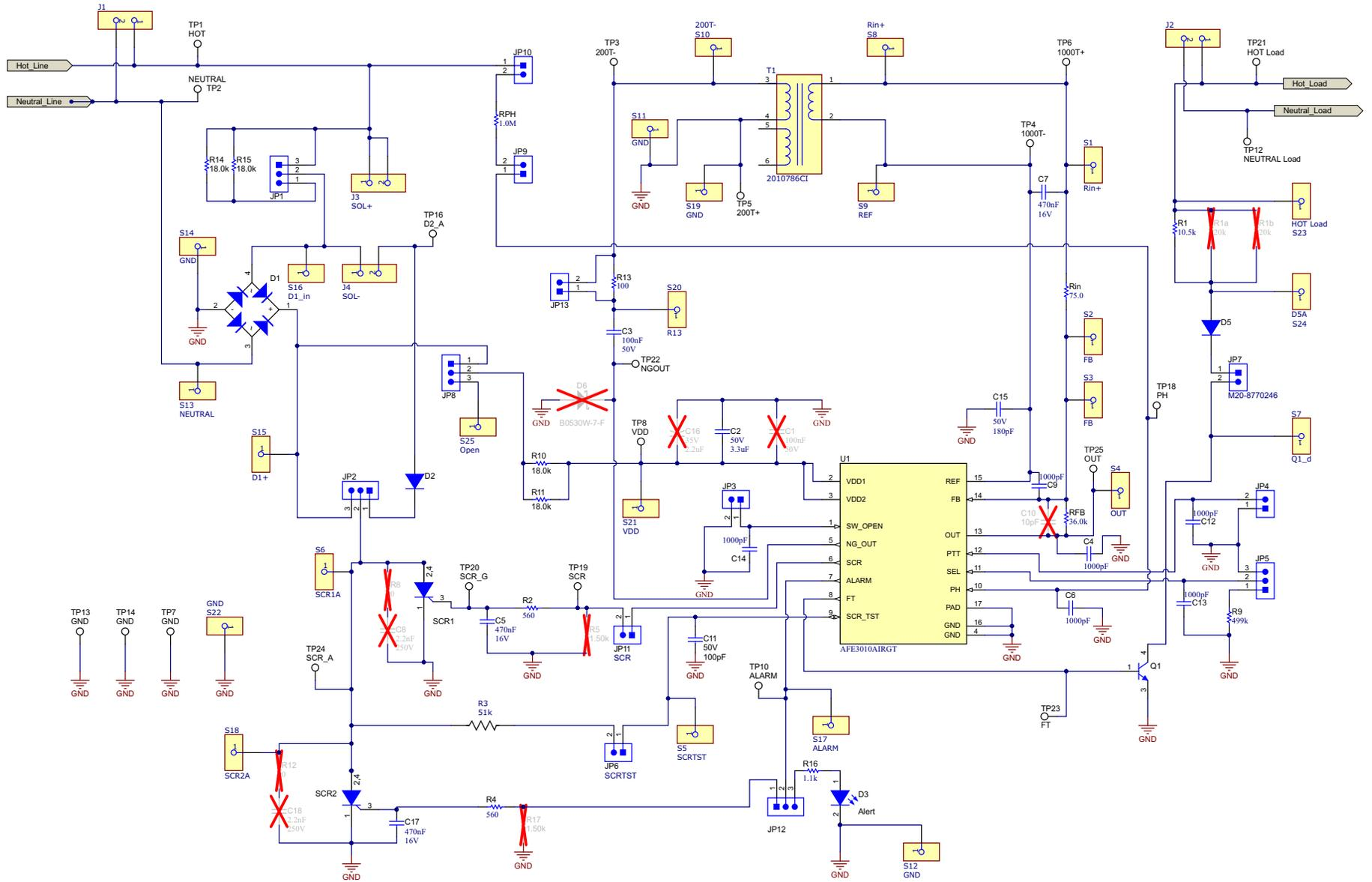
Figure 4. AFE3010EVM Schematic
